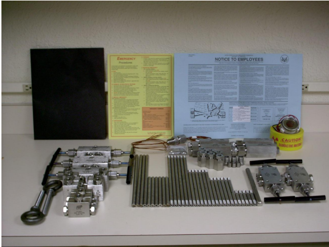
Figure 26 – High Pressure Connections and Valves; Safety Forms
