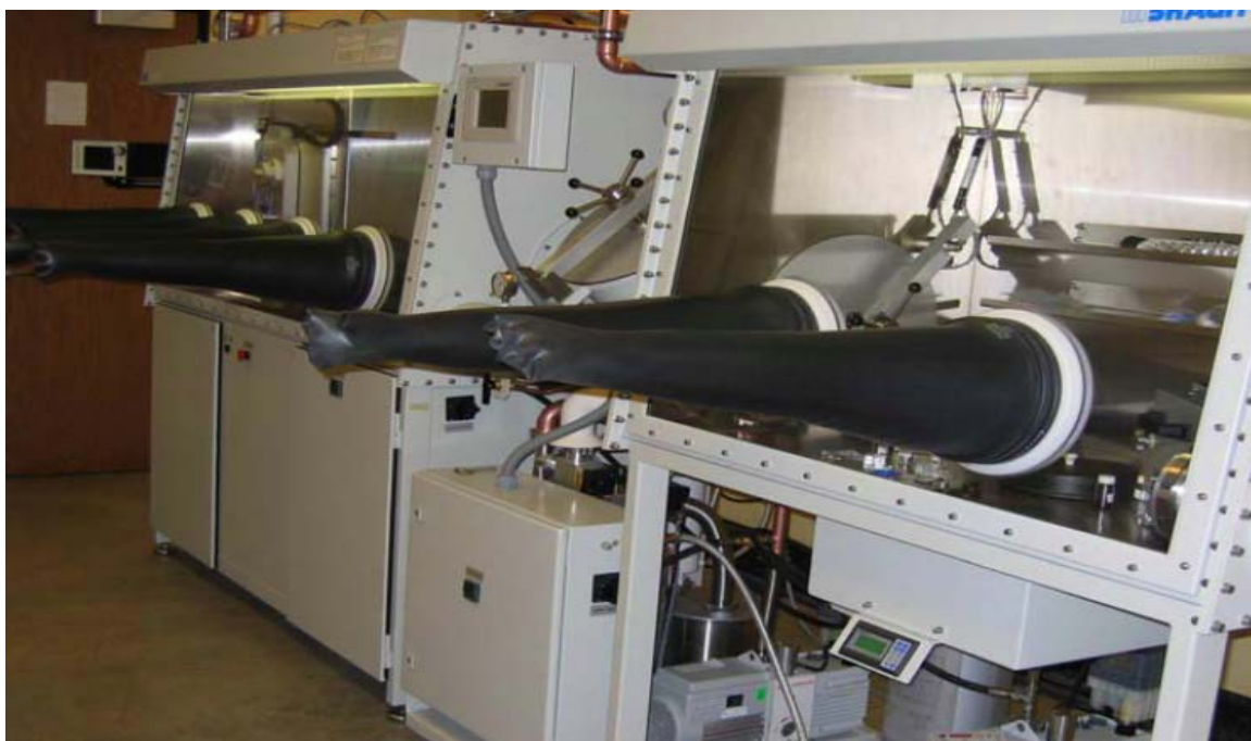
Fig. 3.5: MBraun glove box system with thermal evaporator in box 1 (left).
