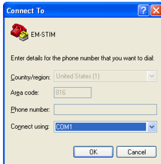
Figure 20: HyperTerminal new connection setup – connect to dialog.
