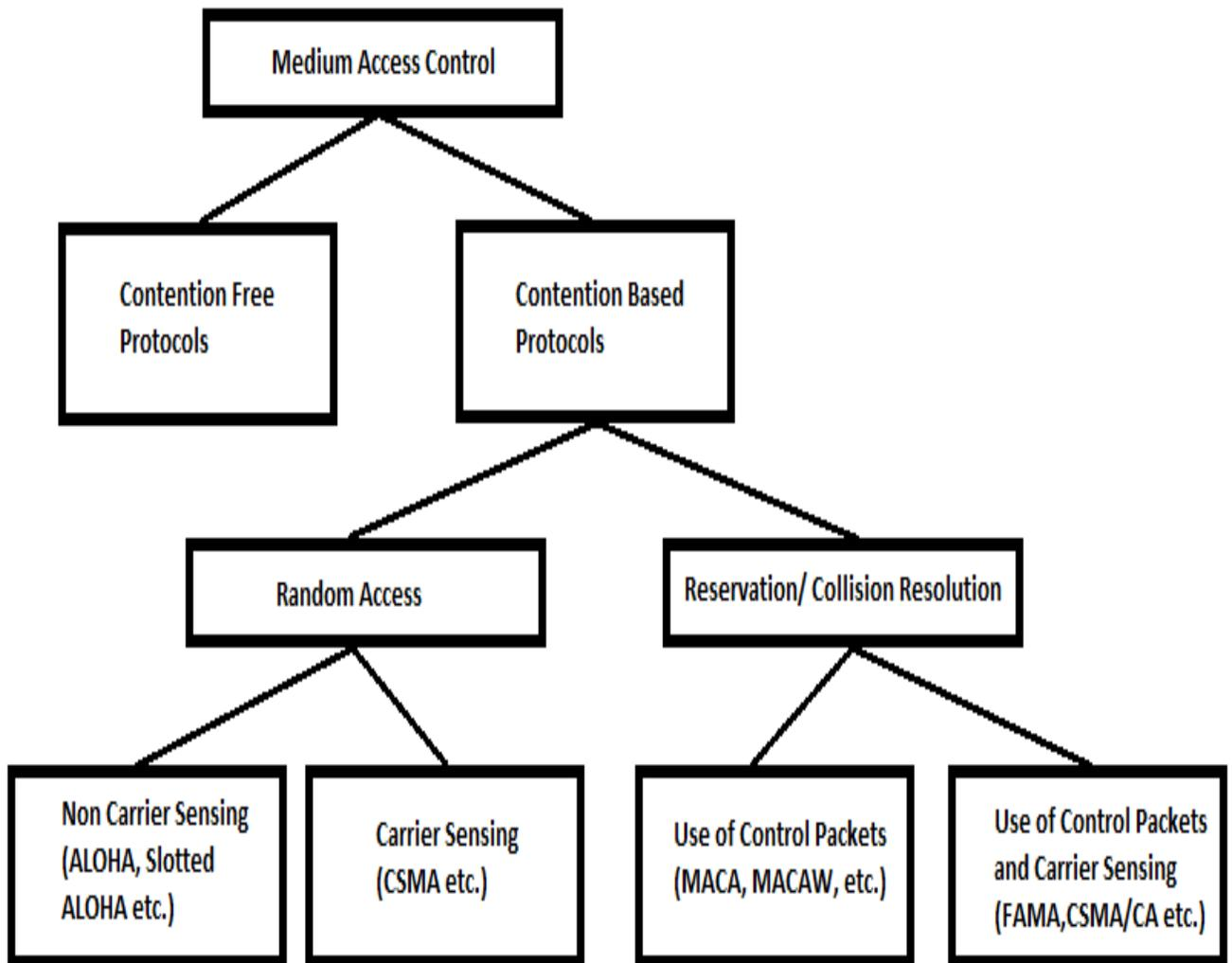
Fig 1.1 Classification of MAC Protocols used for Wireless Ad-Hoc Networks [5]
