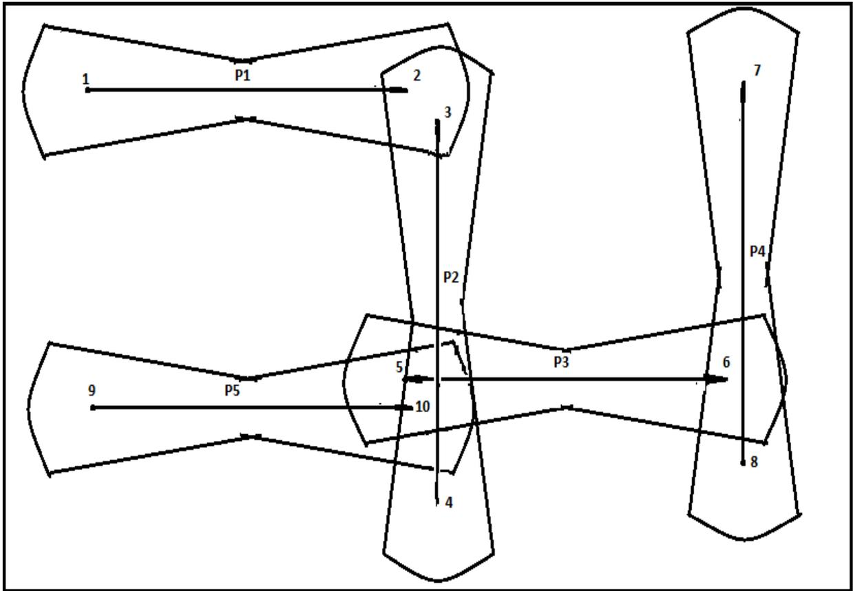
Fig 2.1 Sample Wireless Ad-Hoc Network using Directional Antenna
