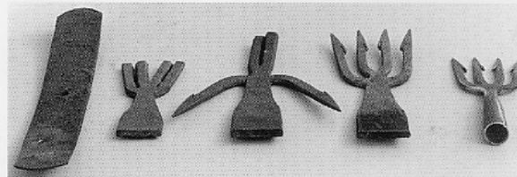
The process of making a four pronged gig is illustrated here. From the collection of Ray Joe Hastings
