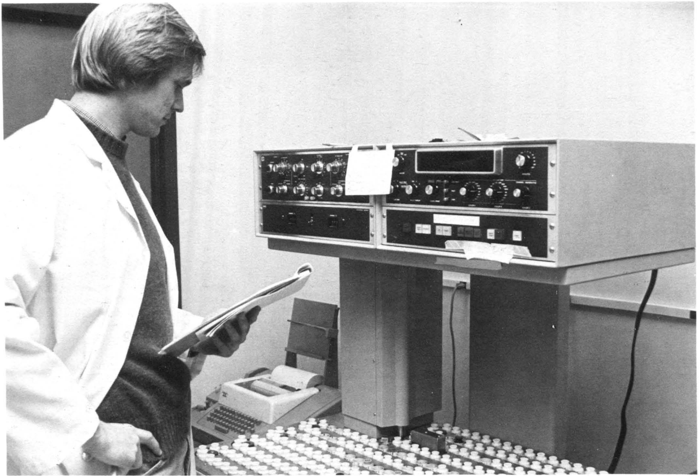
Tom Eschenroeder checks work on the Gamma Counter, a scintillation counter for radioactive assays used in hormonal quantitation.
