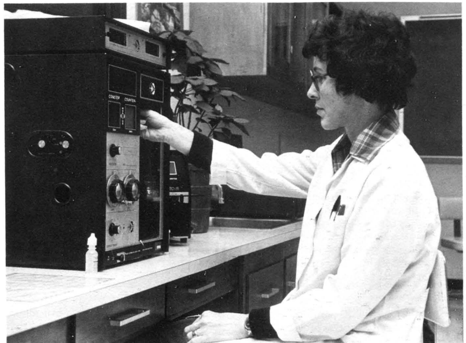
Joanne Adams makes an adjustment on the Coulter Counter, an automatic cell counter used in hematology work.
