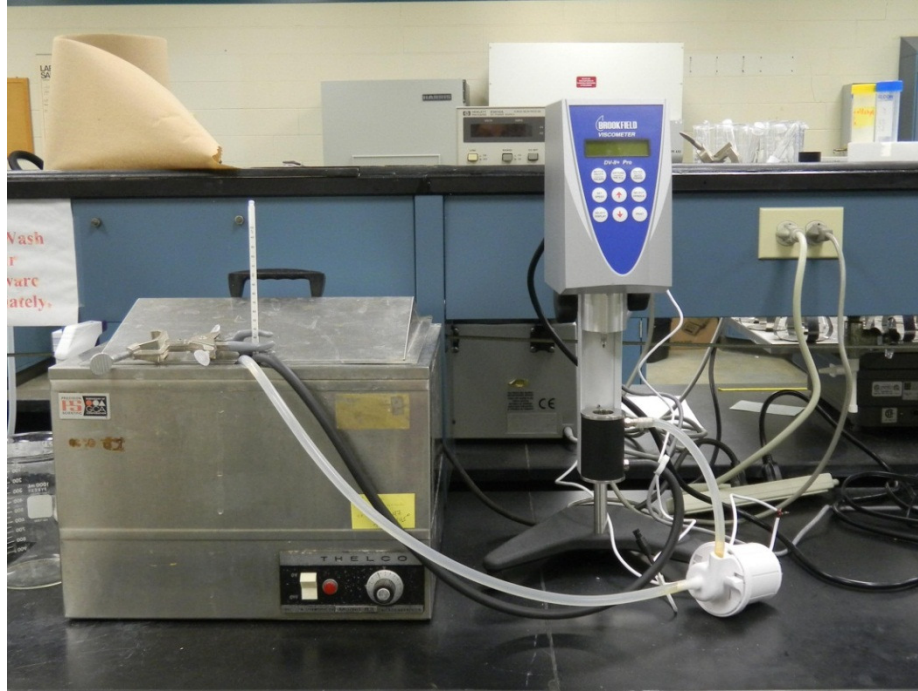
Figure 4.1: Viscometer Testing Set-Up
