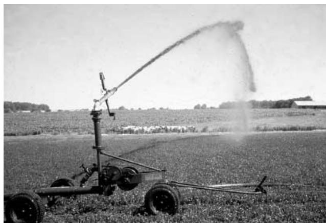
Figure 5. Traveling guns are a common means of irrigating lagoon effluent onto fields.
