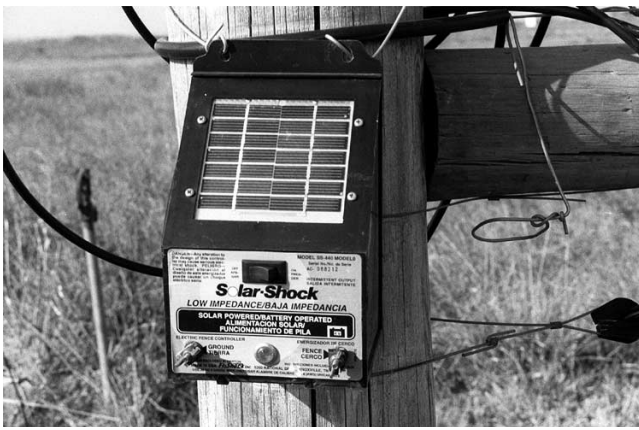
Figure 2. Solar-powered fence energizers use a solar panel to charge a battery.
