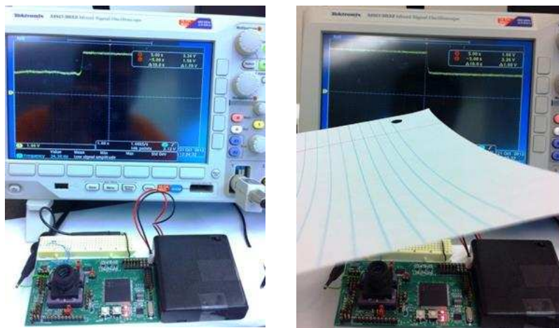
Figure 31: The analog output voltage proportional to the photo-generated current: the output voltage varies with light intensity levels.
