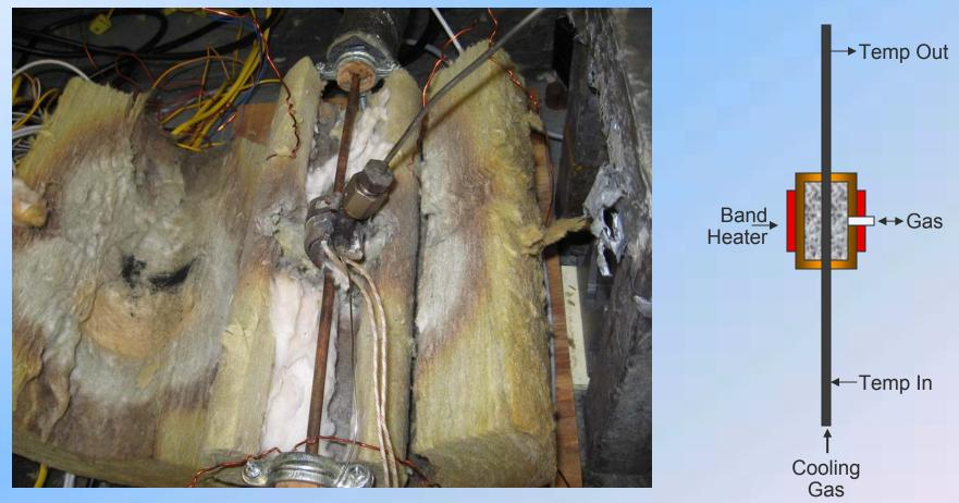
Yan Kurochov, "Method and Apparatus for Energy Generation", WO 98/15986 ➡Theory requires large thermal gradient
