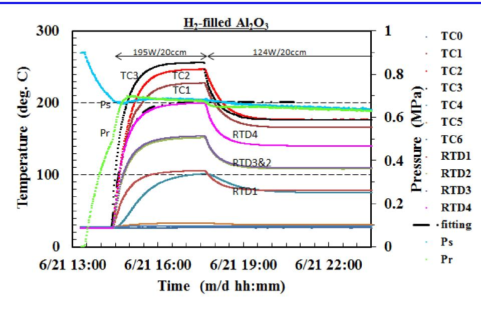
Calibration / control run using Al<sub>2</sub>O<sub>3</sub> powder
