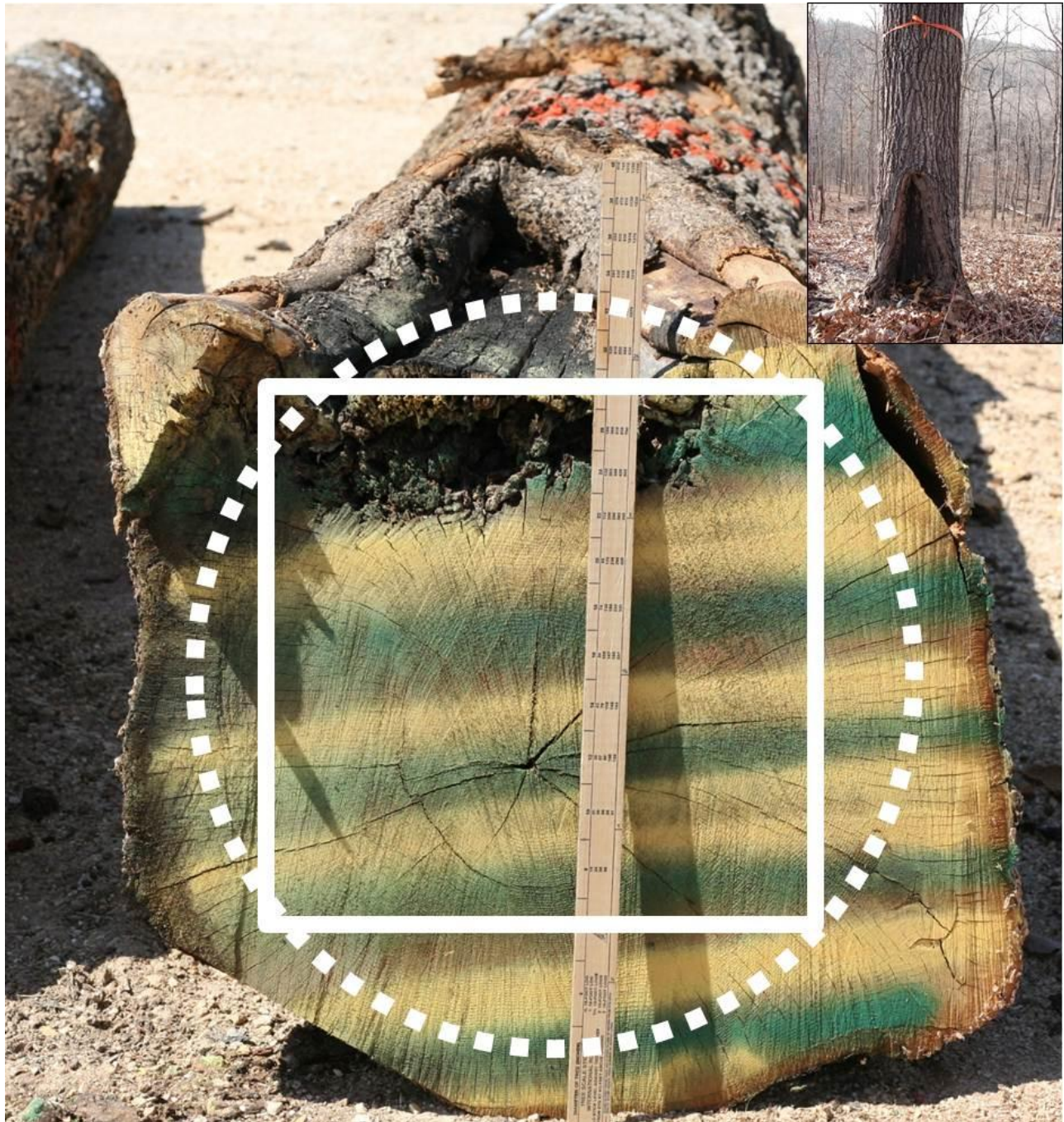
Figure 17. View of base of butt log. Dotted circle approximates the small end diameter, solid square represents the portion of the round log that is utilized when manufacturing rectangular dimensional lumber. Inset (top right) shows the tree prior to cutting.
