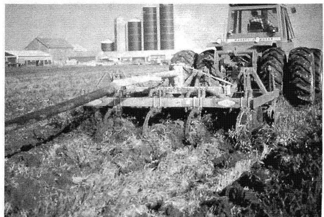
Figure 12. Injection of solids reduces odors and helps retain fertilizer nutrients.
