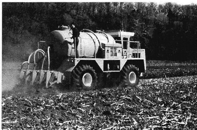
Figure 3. Tank trucks with injector units are used to land-apply solids slurry beyond pumping distance from the lagoon.
