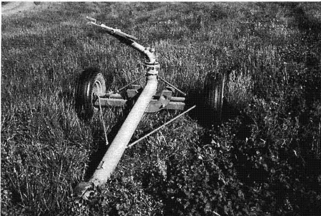
Figure 10. Cable-tow traveling guns are fed by a flexible hose, which drags behind the gun.
