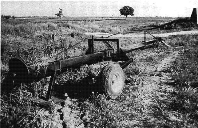
Figure 4. A wheel-mounted, PTO-driven propeller/agitator is used to stir and suspend solids in a lagoon.
