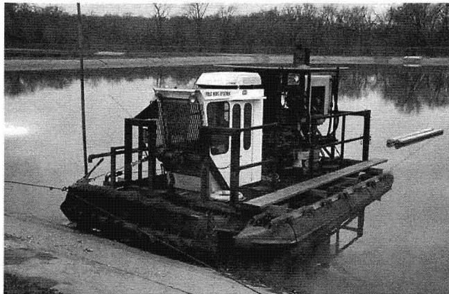
Figure 1. Dredge used to remove solids from municipal and industrial lagoons.
