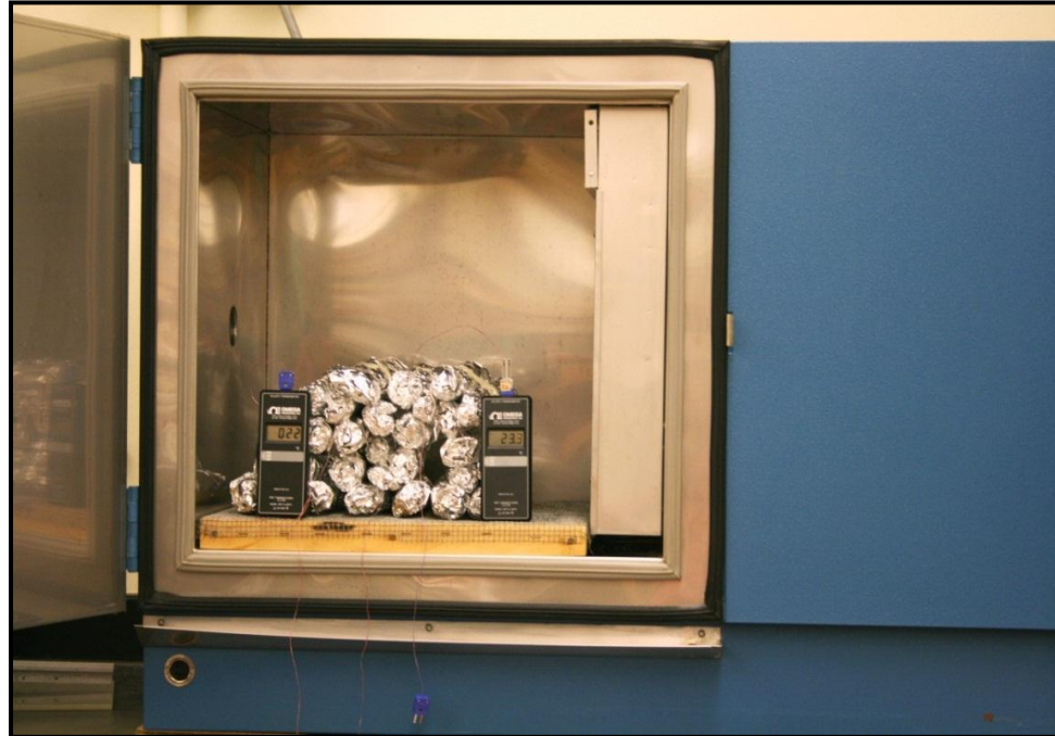
Fig. 3. Bundles of wrapped budsticks with thermocouples attached to digital thermometers in the programmable chamber before a freezing test was conducted.
