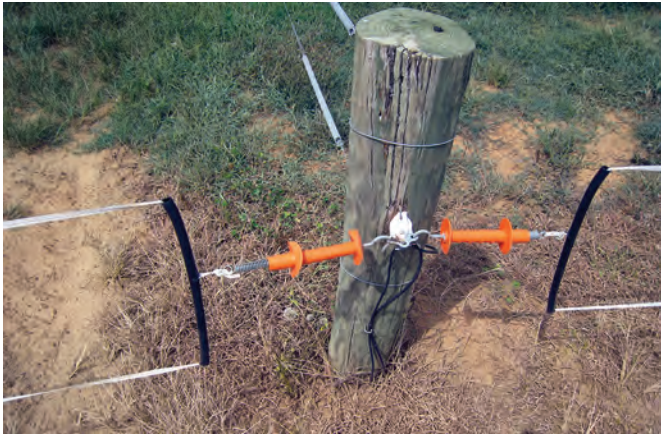
Figure 11. An insulated gate handle with an extension spring provides leeway in fitting the opening.
