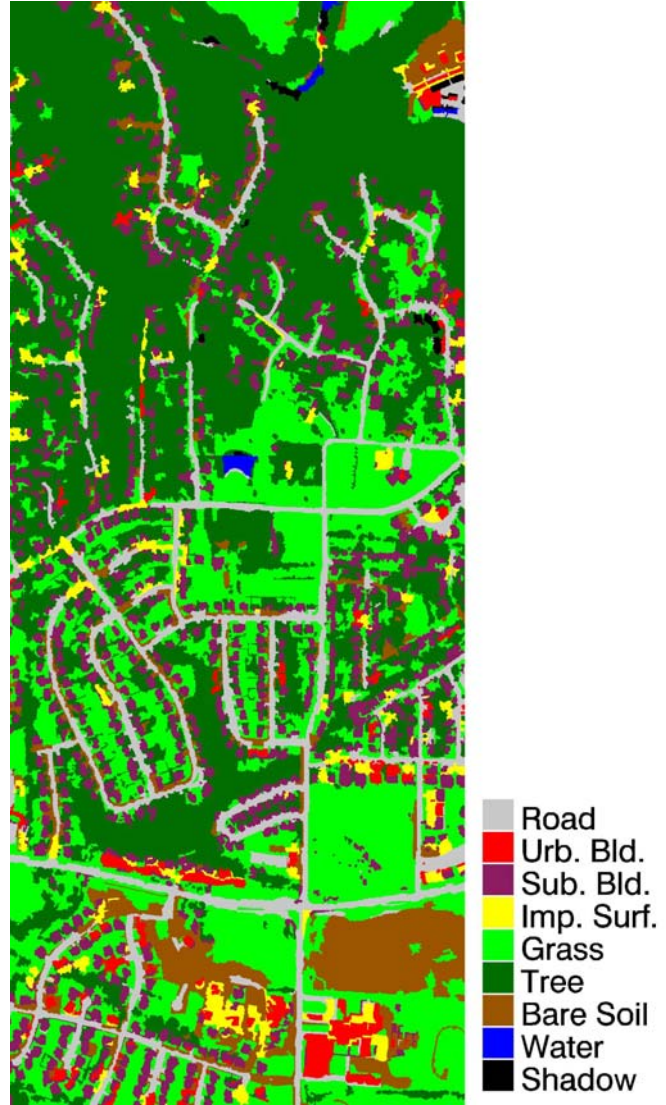
Figure 3-10. Fuzzy logic object-based classification of suburban area shown in Fig. 3-9 with differentiation between urban and suburban buildings.
