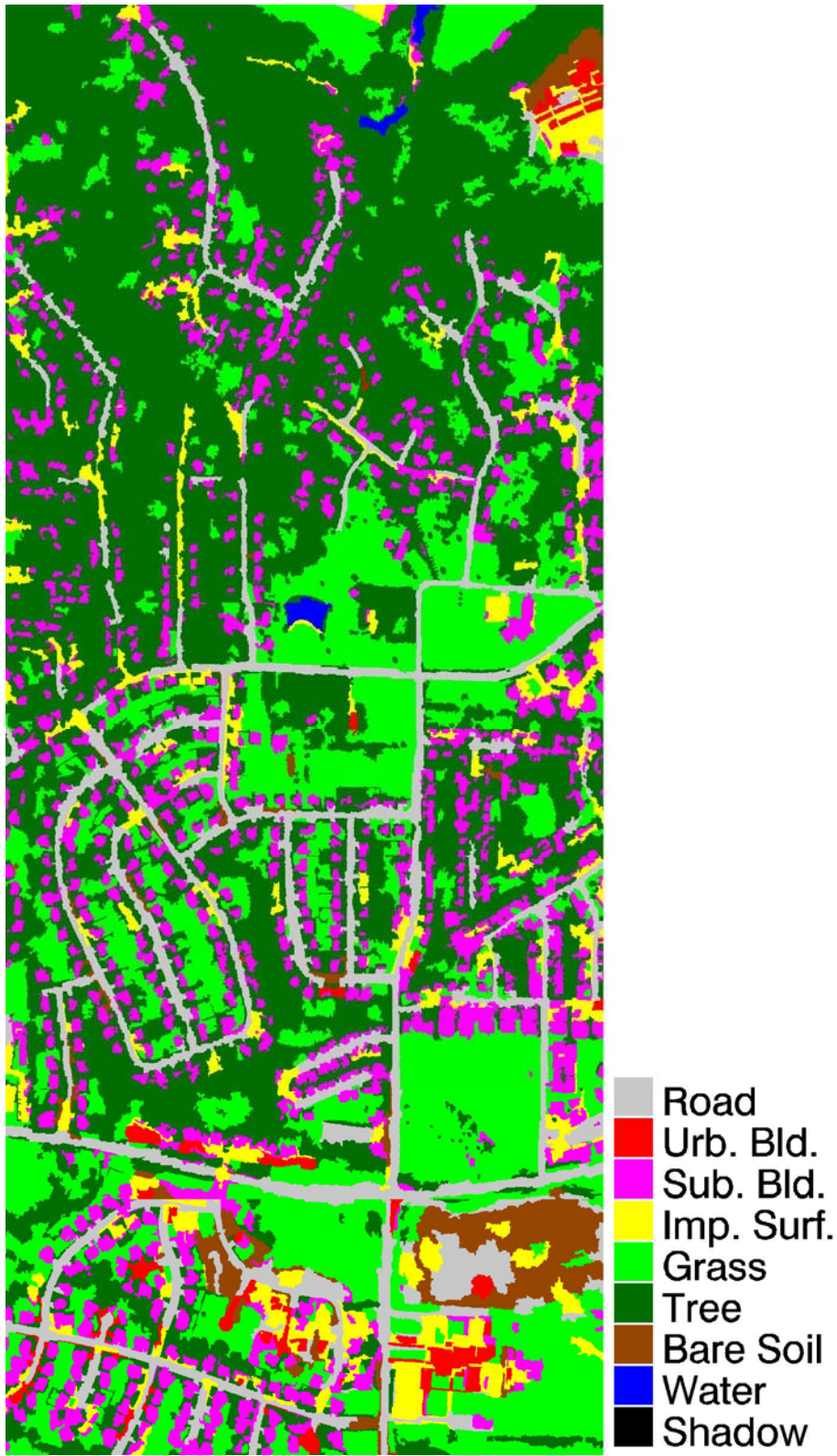
Figure 6-7. Self-supervised fuzzy logic object-based classification of suburban area shown in Fig. 3-9 with differentiation between urban and suburban buildings.
