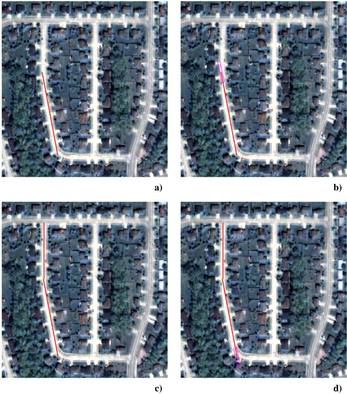
Figure 4-5. Illustration of road segment growth: a) identification of initial road segment, b) examination of length-width values around endpoint 1, c) resulting line segment, d) examination of length-width values around endpoint 2 (no valid line segment identified).
