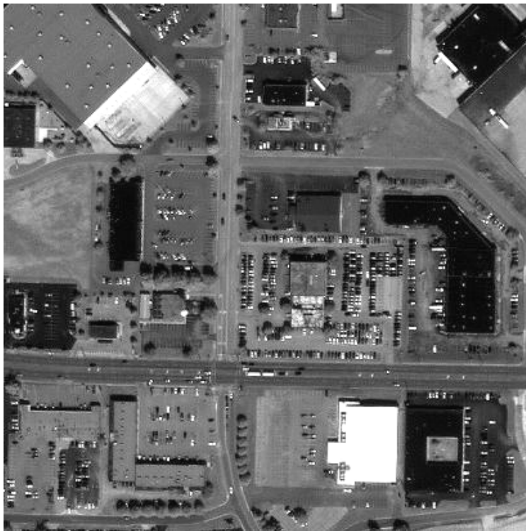
Figure 1-9a. IKONOS PAN image of commercial land use area. Note the difference in image quality between the IKONOS data and the DOQQ image (both 1 m resolution).
