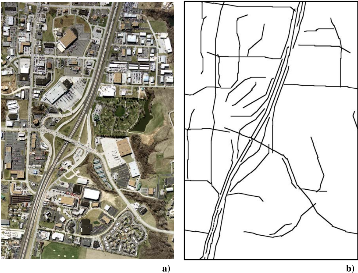
Figure 4-7. Road network extracted from digital orthophoto by fully automated algorithm. a) commercial/industrial test site, b) extracted road network.
