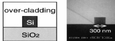
Figure 62. Optical waveguide by SOI method [37].
