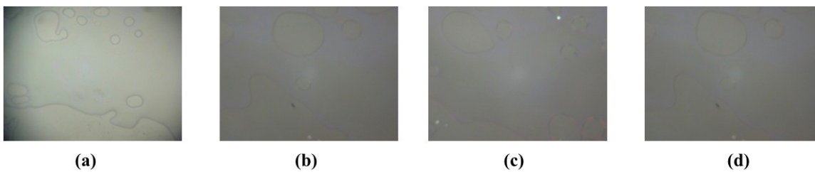
Figure 1.24. Polarized optical microscopy images of compound 1c in heating process at 25 °C (a), at 75 °C (b), and cooling process at 45 °C (c), at 27 °C(d).
