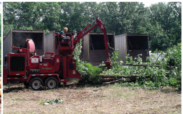
Figure 7. An integrated, one-pass harvest sorts and processes low-value woody biomass at the landing.
