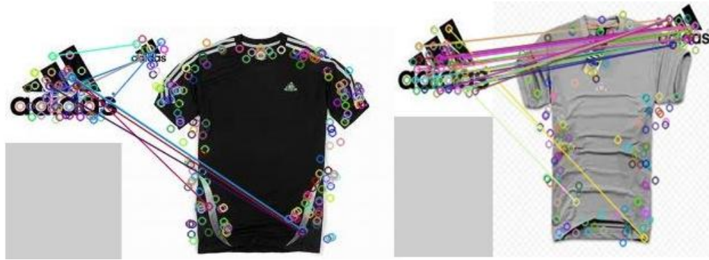
Figure 3.15 Phase 3: SURF Image Processing Output
