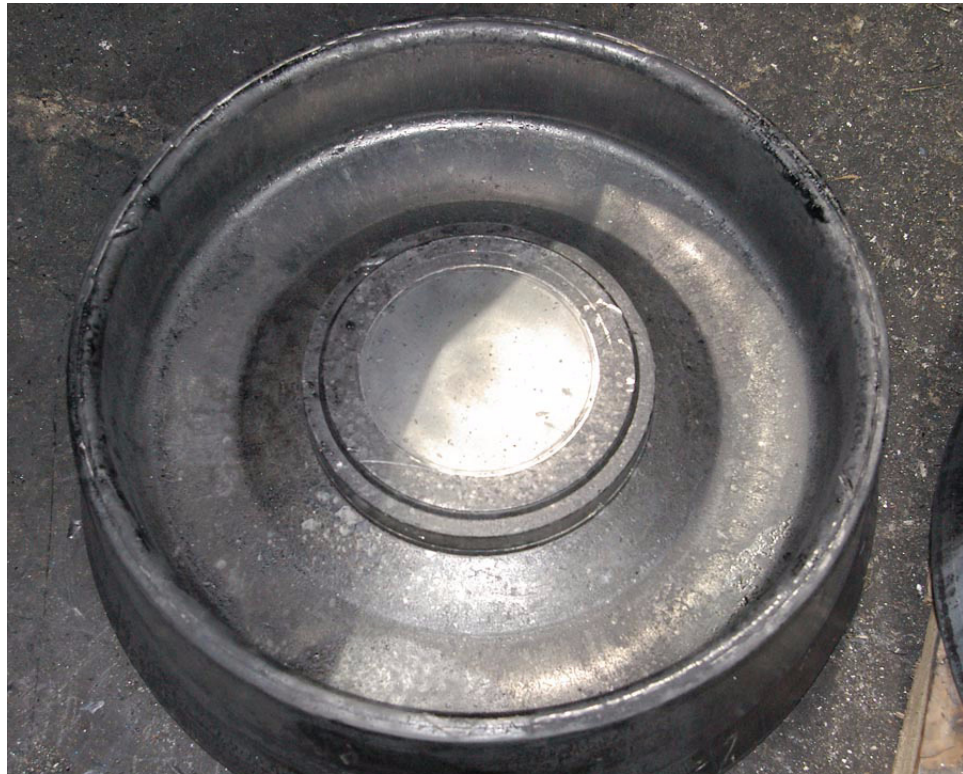
FIGURE 168. Bottom view of billet after forging.
