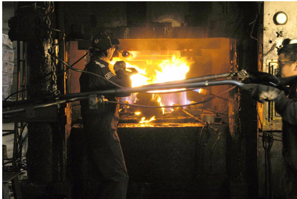
FIGURE 166. Lubricant application and excessive flashing produced.
