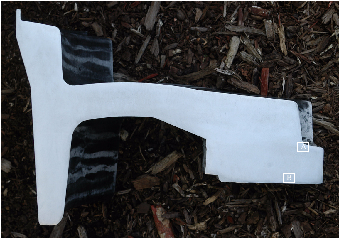
FIGURE 172. Half crosssection of billet after completion of forging operation, polished and then etched using Tucker's reagent. Metallurgical samples removed from areas A and B.
