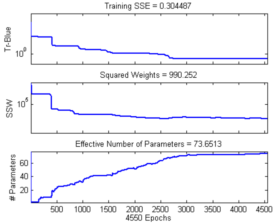
FIGURE 84. Progression of training using normalized values of \ln(\text{strain}) , \ln(\text{strain rate}) , 1/\text{temperature} , \ln(\text{stress}) with 10-3 neurons, BR training algorithm.
