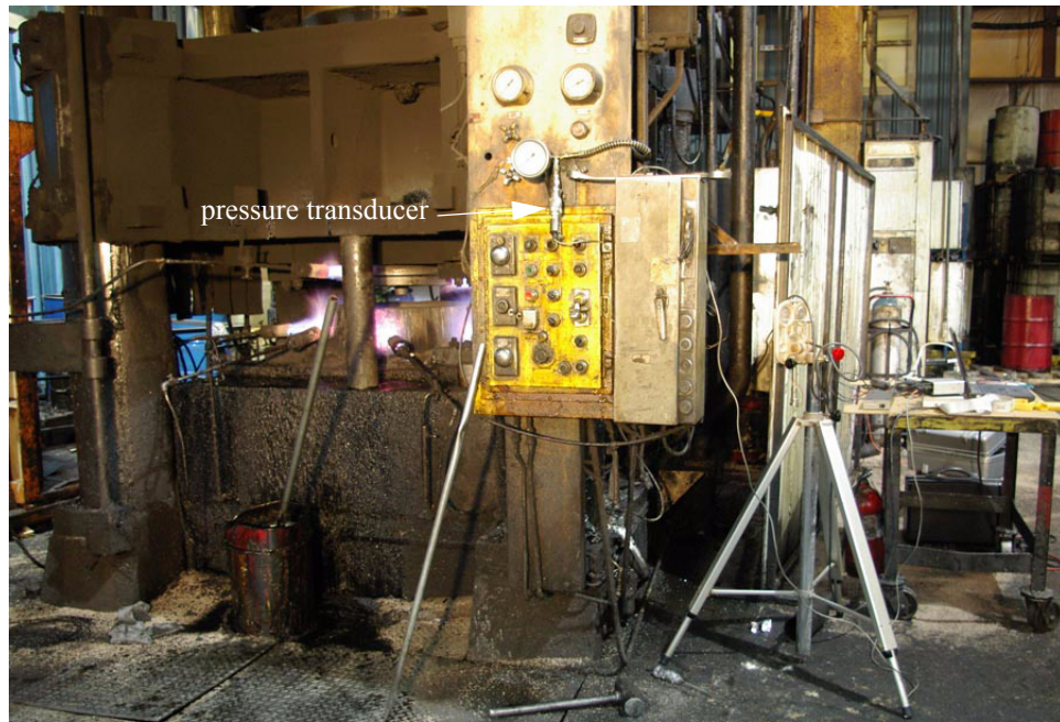
FIGURE 163. View showing front of the forging press and pressure transducer.
