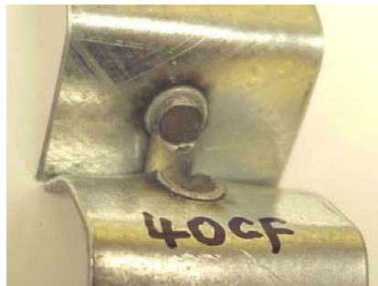
Figure 6.12 HSLA340Y GI coach peel sample fatigue failure at of 5,103 cycles (5X)
