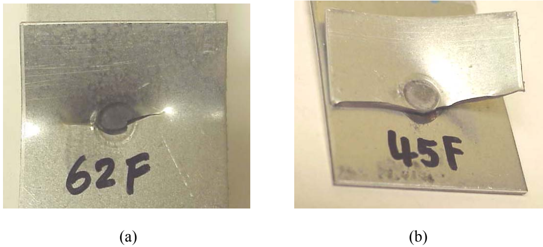
Figure 6.7 DP600 GI tensile shear fatigue sample failure modes: (a) with fatigue of 55,350 cycles, and (b) 2043,850 cycles.
