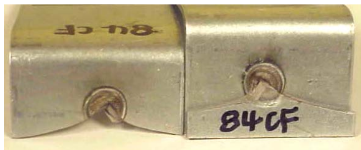
Figure 6.13 DP600 GI coach peel fatigue sample failure modes: (a) with fatigue of 995 cycles, and (b) 1524,765 cycles.
