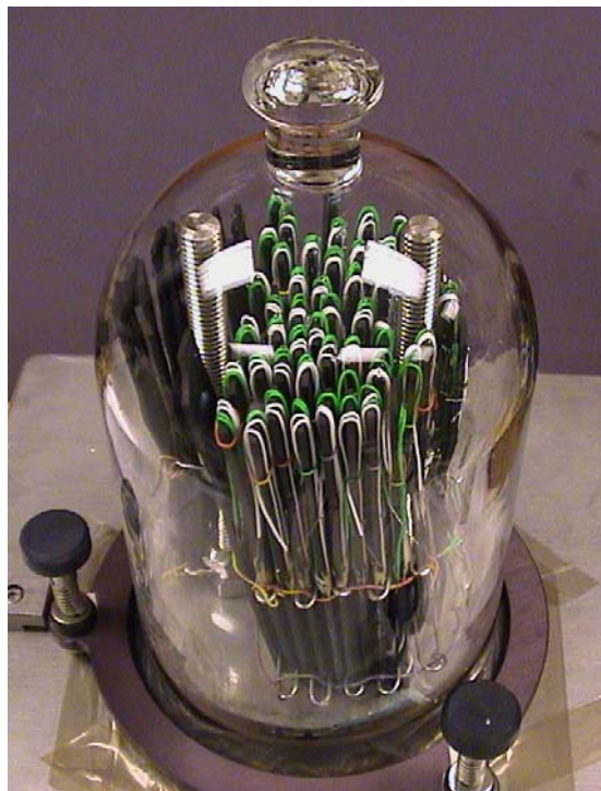
Figure 5-12. Composite specimens loaded in the conditioning chamber.
