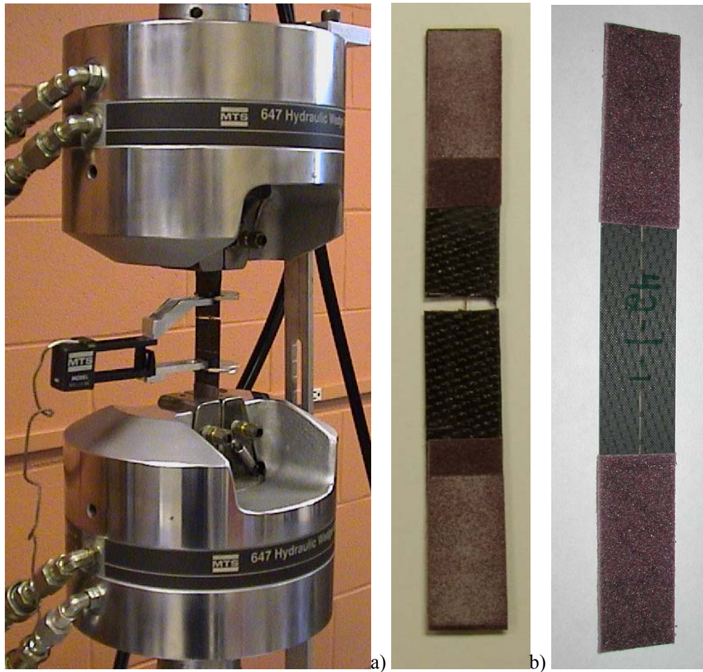
Figure 6-4. Tension test setup for composite sample, note the emery cloth extends past the grips approximately 12.5 (0.5 in). The sample is shown again in b); the light colored portion of the emery cloth was the area inside the grips. A new sample is shown in c).
