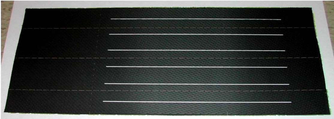
Figure 5-8. Lateral lines being cut in the composite panel.
