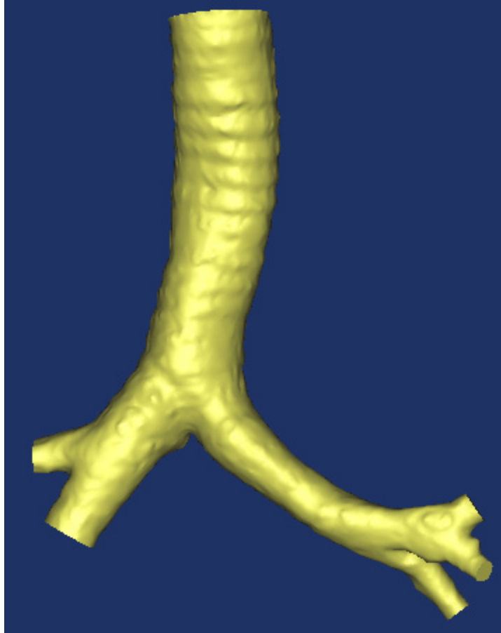
Figure 6.12: Simplified geometry after cutting and removing the end bifurcations on the geometry in Figure 6.5 (b)
