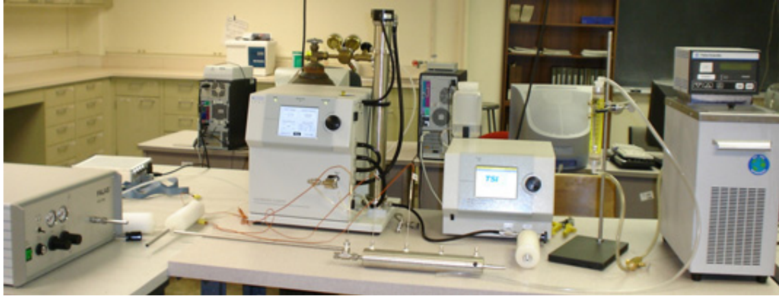
Figure 3.14: Complete experimental setup for thermophoretic deposition of particles that includes a particle generator GFG-1000, electrostatic classifier, ultrafine condensation particle counter, water bath chiller and thermophoretic deposition tube assembly.
