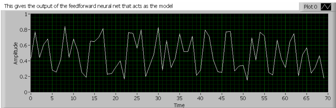
Fig. 5.38 Output of the FF neural network with 5 input neurons, 20 hidden neurons & 1 output neuron which is trained for 300 epochs. The first 70 data points have been used for training and testing. Learning Rate = 0.2
