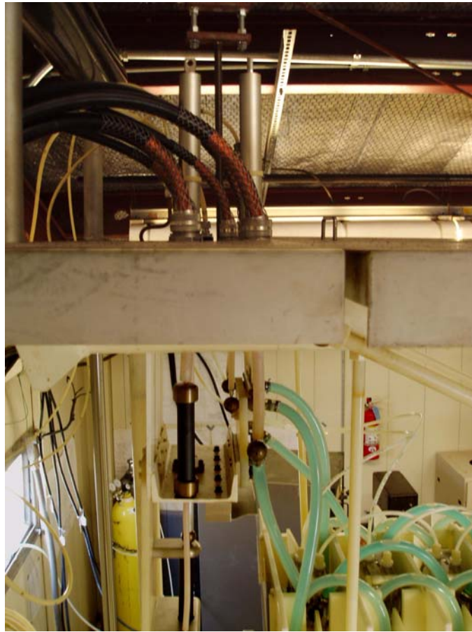
Figure 2.14. Crowbar assembly with input charging and triggering lines
