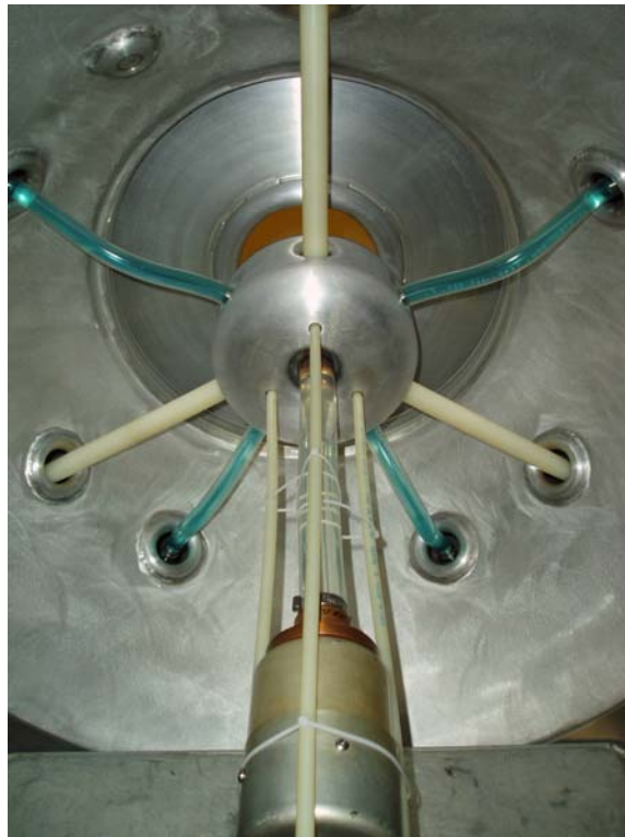
Figure 3.5. Post-switch voltage divider
