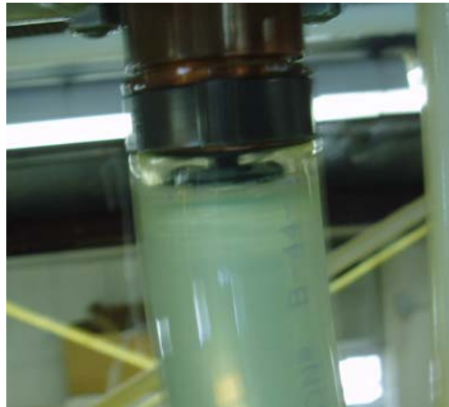
Figure 3.3. Voltage divider middle electrode
