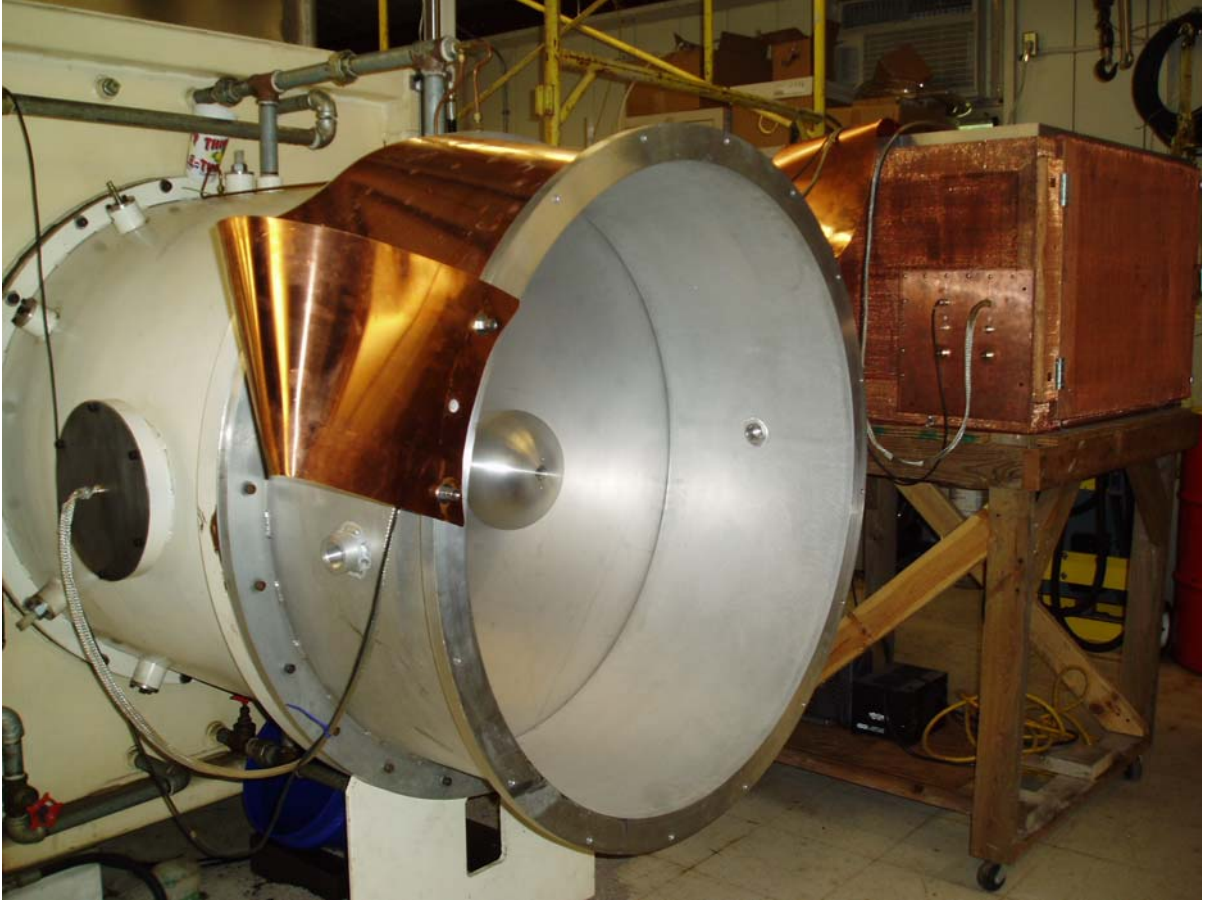
Figure 3.11. Diagnostic output connections and Faraday cage
