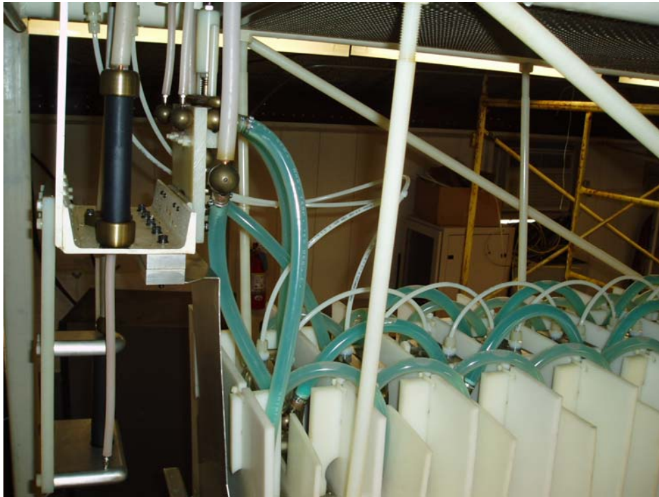
Figure 2.8. Charging and triggering resistors
