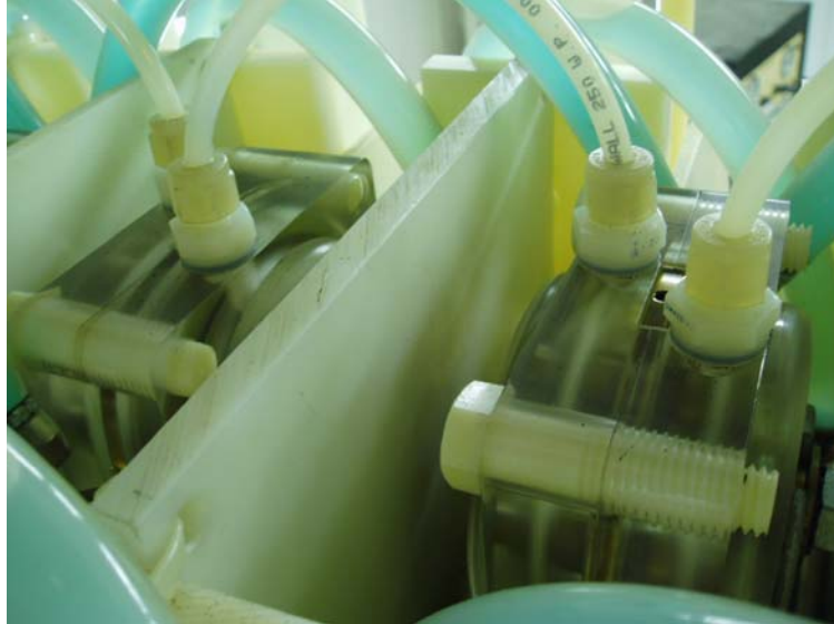
Figure 2.10. Spark gaps installed in Marx
