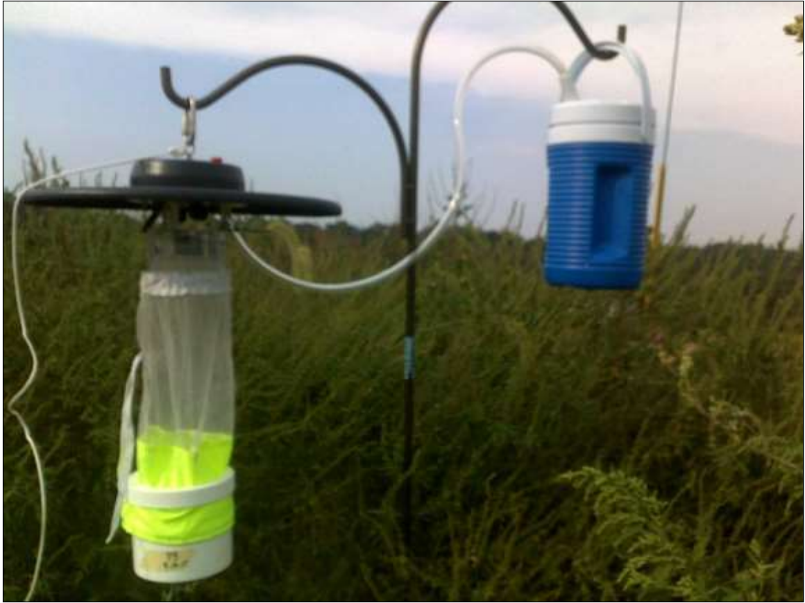
Figure 16 CDC Miniature light trap used at all collection sites. Dry ice was used as an attractant for mosquito collection. Host-seeking females were drawn into the collection cup when attracted to carbon dioxide emitted from hose.
