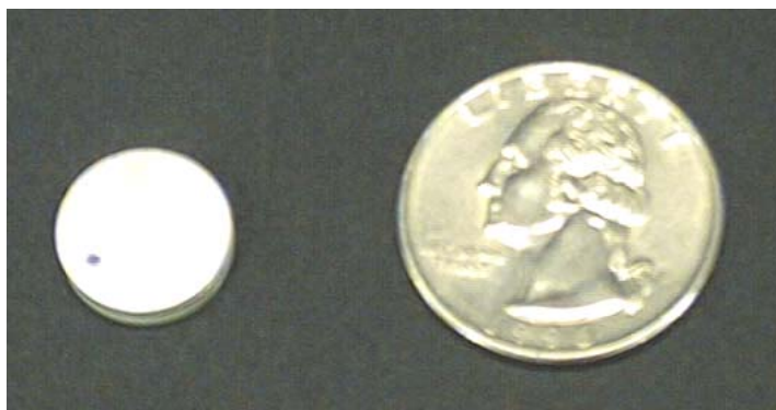
Figure 1. Photograph of single piezoelectric element showing relative size. Positive polarity side of element is identified with a black dot.
