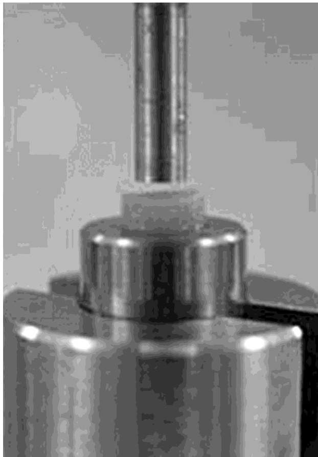
Figure 5-1. Custom made stainless steel fixtures consisting of the impactor ( \phi = 3.9\text{mm} ) attached to test machine ram (A), well ( \phi = 6.01\text{mm} ) (B), and base fixture (C) attached to test machine table used to measure the thickness and deliver impact injury of an osteochondral explant ( \phi = 6\text{mm} , thickness= 3.6\pm 0.29\text{mm} ) (D).
