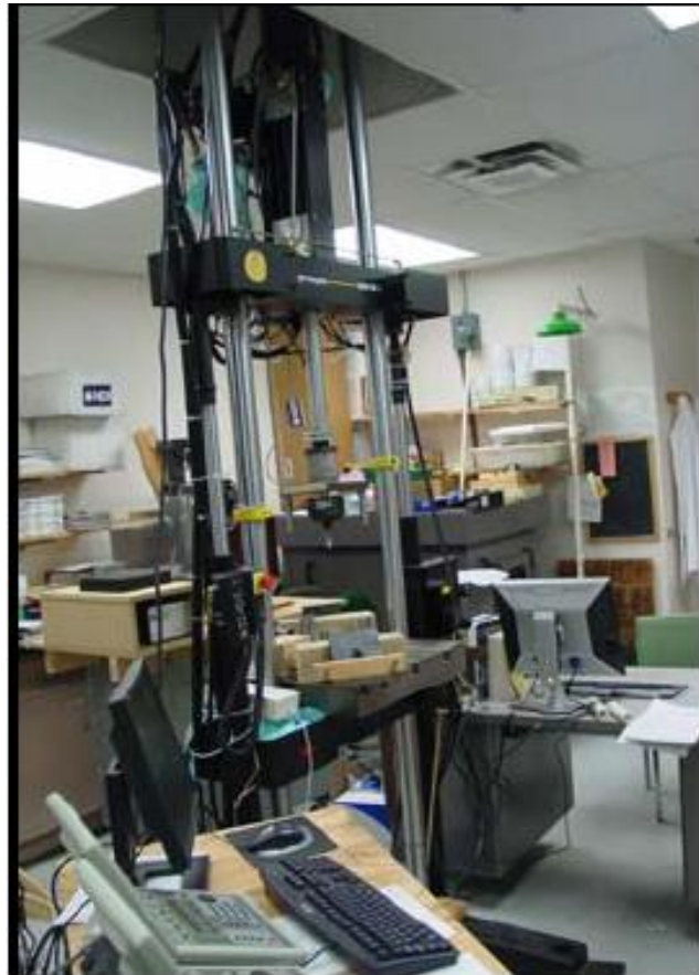
Figure 2-11. Instron 8821s servo-hydraulic testing machine in the biomechanics lab of the Comparative Orthopaedic Laboratory (COL). For this project, the machine was equipped with a 1000 N load cell attached to the ram which has a maximum ram travel of 260 mm. A stainless steel impactor (tip diameter of 3.9 mm) attached to the end of the ram (below the load cell) and a stainless steel base (containing a stainless steel anvil with specimen-restraining well located in the center) was attached to the test table (See Appendix B for detailed fixture drawings).
