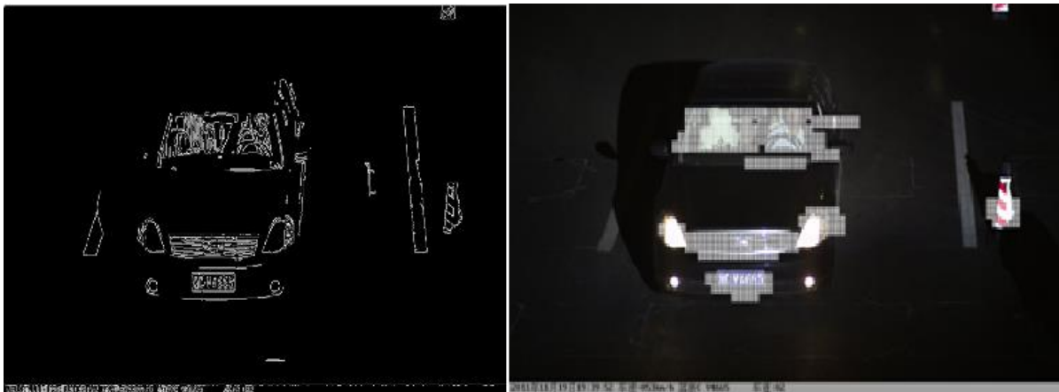
Fig. 2. 9. Using Edge information. (a) The canny edge image; (b) The scanning regions that will be classified by SVM.
