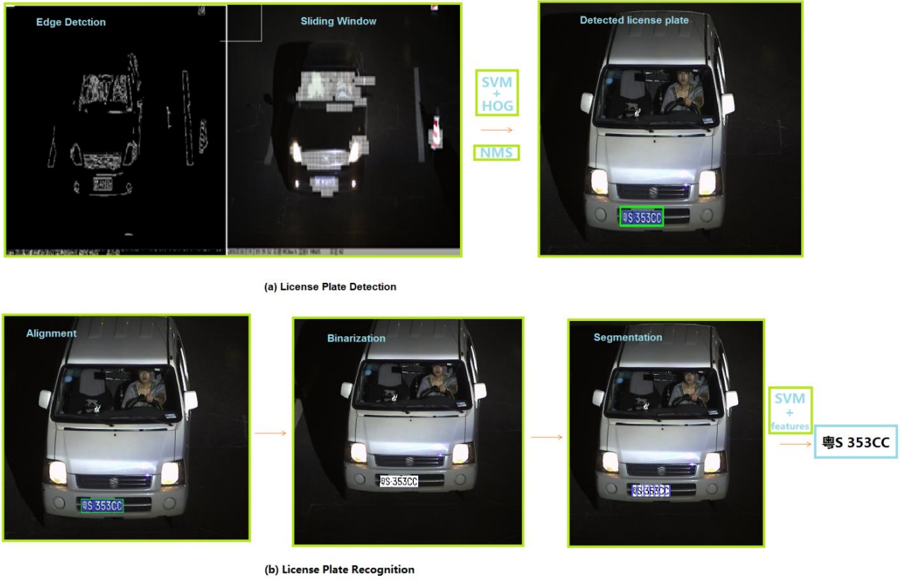
Fig. 1. 2. Overview of our proposed method. (a) Shows the procedure of license plate detection; (b) shows the procedure of license plate recognition
