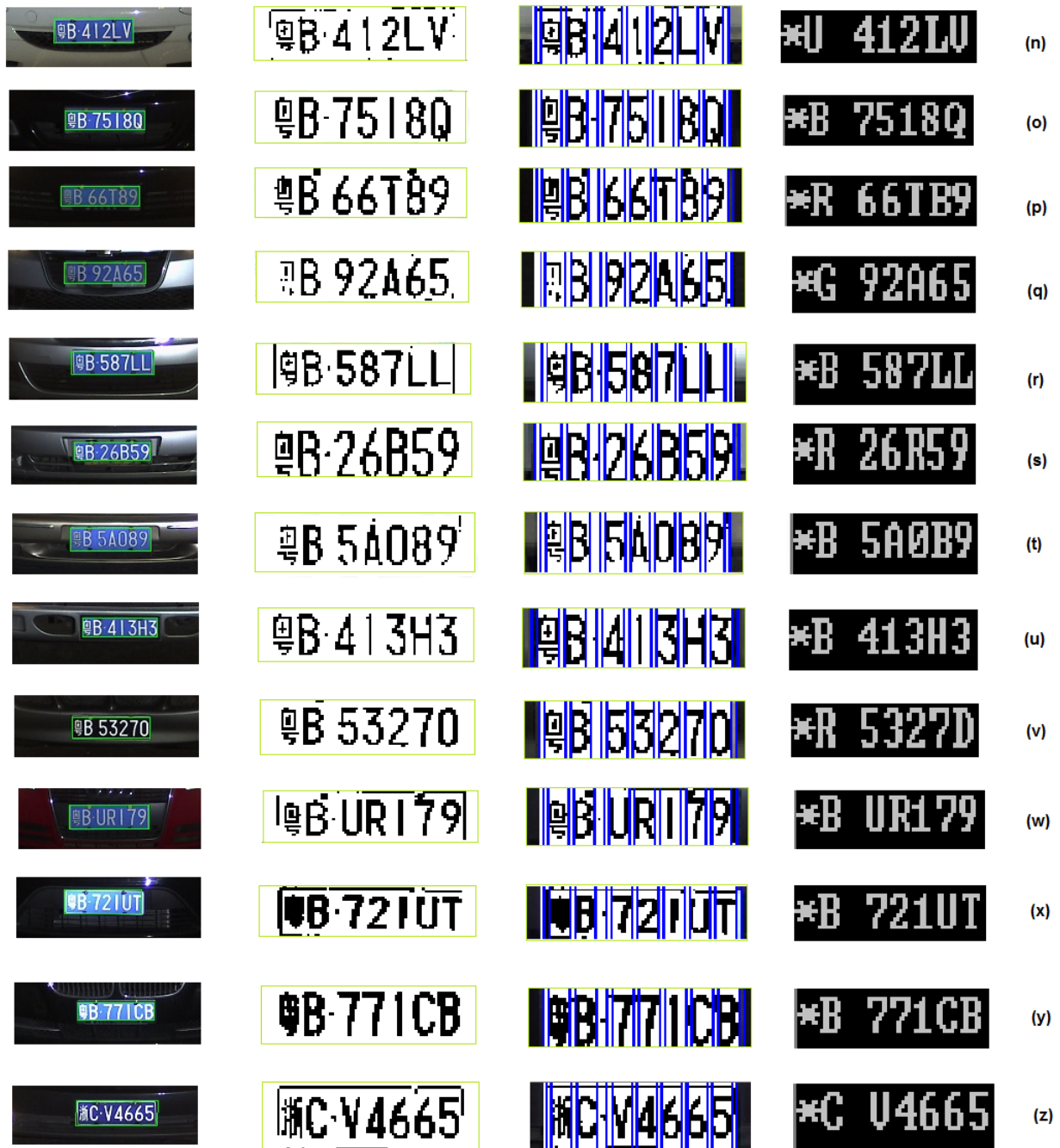
Fig. 3. 22. Sampled results of global alignment, k-means binarization, segmentation and character recognition. The recognition part ignores Chinese characters and output a "*" instead.
