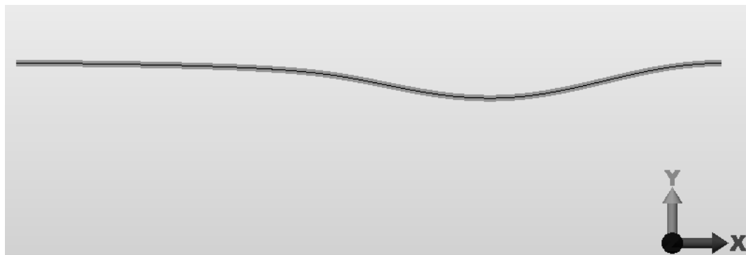
Figure 3.7 Buckling mode for load applied at a distance x = 0.45 in (19 th node)
