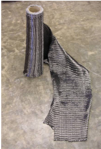
Figure 2-9 - Wet-layup FRP arrives at the jobsite on rolls.
