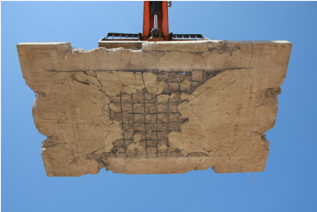
Figure 2-5 – Un-strengthened reinforced concrete slab after blast at a scaled range of 1.5 \text{ ft/lb}^{1/3} , displaying extensive spalling.
