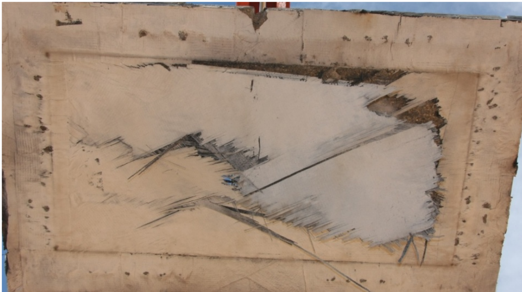
Figure 2-25 – CFRP mitigated slab subjected to a close-in blast at a scaled range of 1\text{ft}/\text{lb}^{1/3} (Orton 2013).
