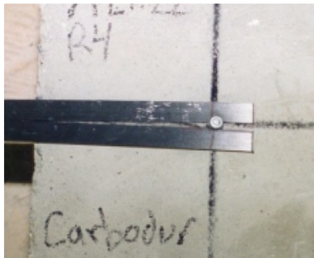
Figure 2-20 – Splitting occurs around mechanical fasteners in pultruded CFRP without cross fibers (Lamanna 2002).
