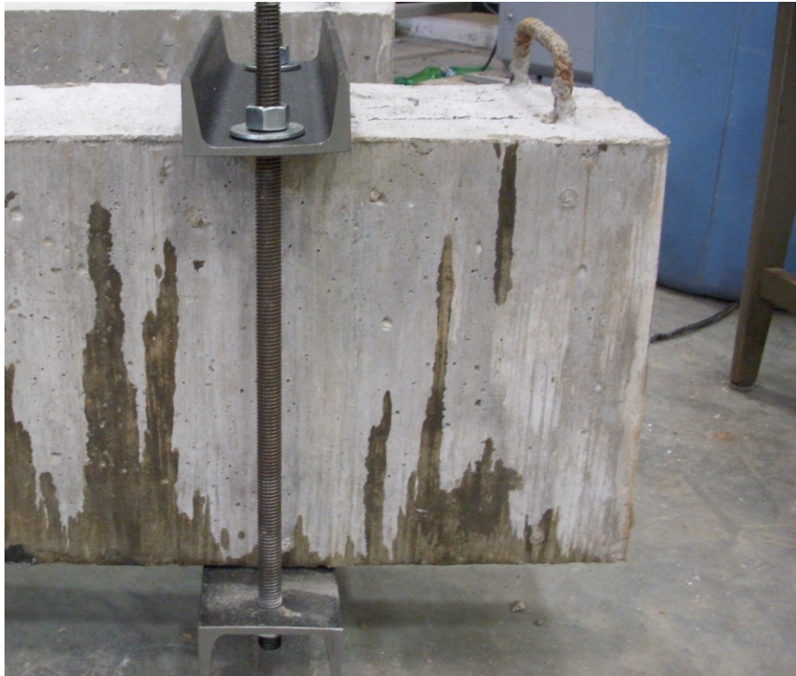
Figure 2-15 - Mechanical clamp anchors used to limit de-bonding of FRP (Orton 2011).
