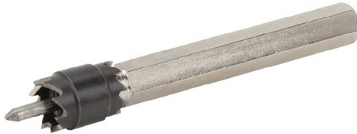
Figure 3-10 – Annular cutter used to drill CFRP. CFRP was found to very rapidly dull, overheat, and clog cutting tools.
