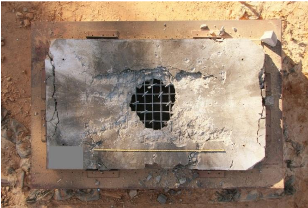
Figure 2-24 – Unmitigated concrete slab tested at a scaled range of 1\text{ft}/\text{lb}^{1/3} (Orton 2013)
