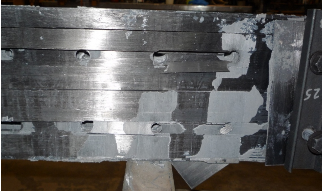
Figure 5-4 - The longitudinal CFRP sheets split next to many of the bolt holes. This may have contributed to extensive slipping of the CFRP sheets.
