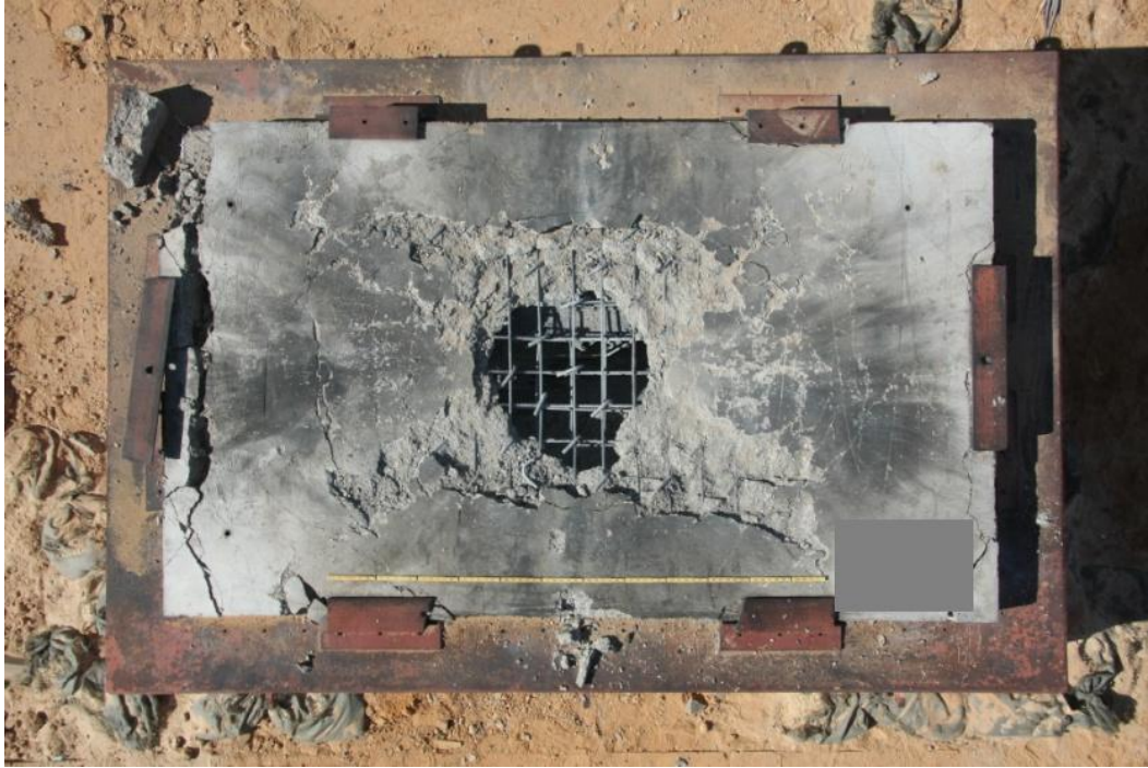
Figure 2-25 – CFRP mitigated slab subjected to a close-in blast at a scaled range of 1\text{ft}/\text{lb}^{1/3} (Orton 2013).
