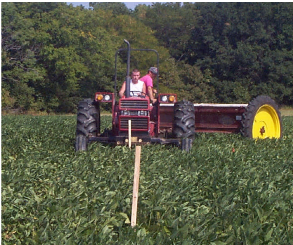
Figure 3. Modified drop seeder used for overseeding annual ryegrass and cereal rye into soybean.
