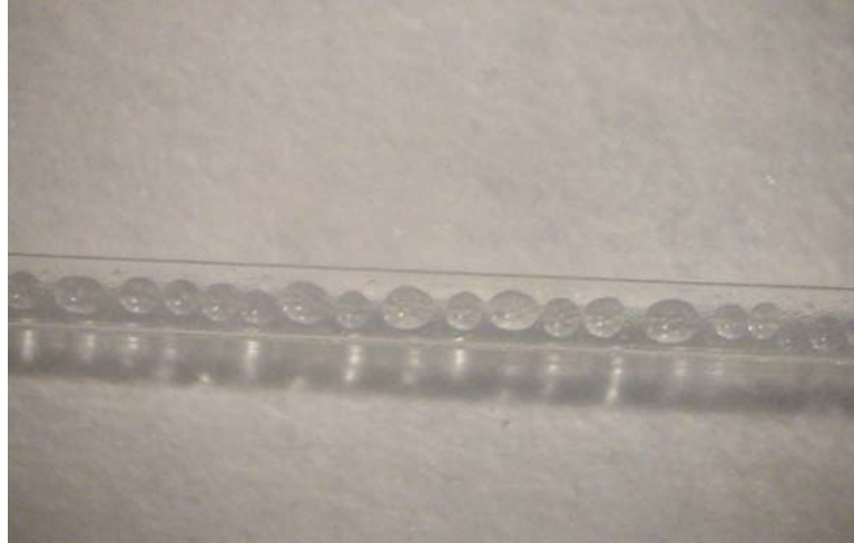
Fig.5.5: Bubbles entrapped in capillaries
