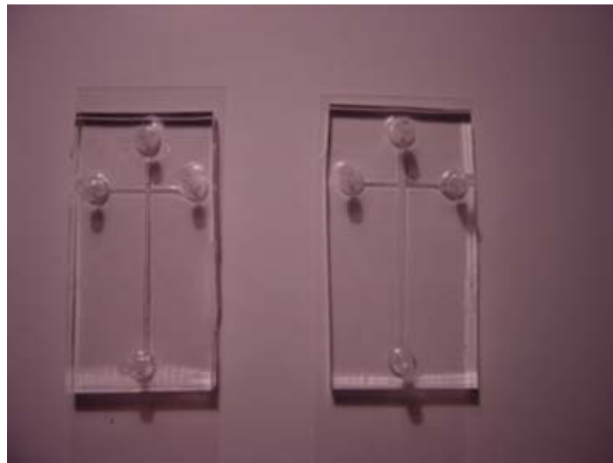
Fig. 5.1: Mask for micro channel electrophoresis
