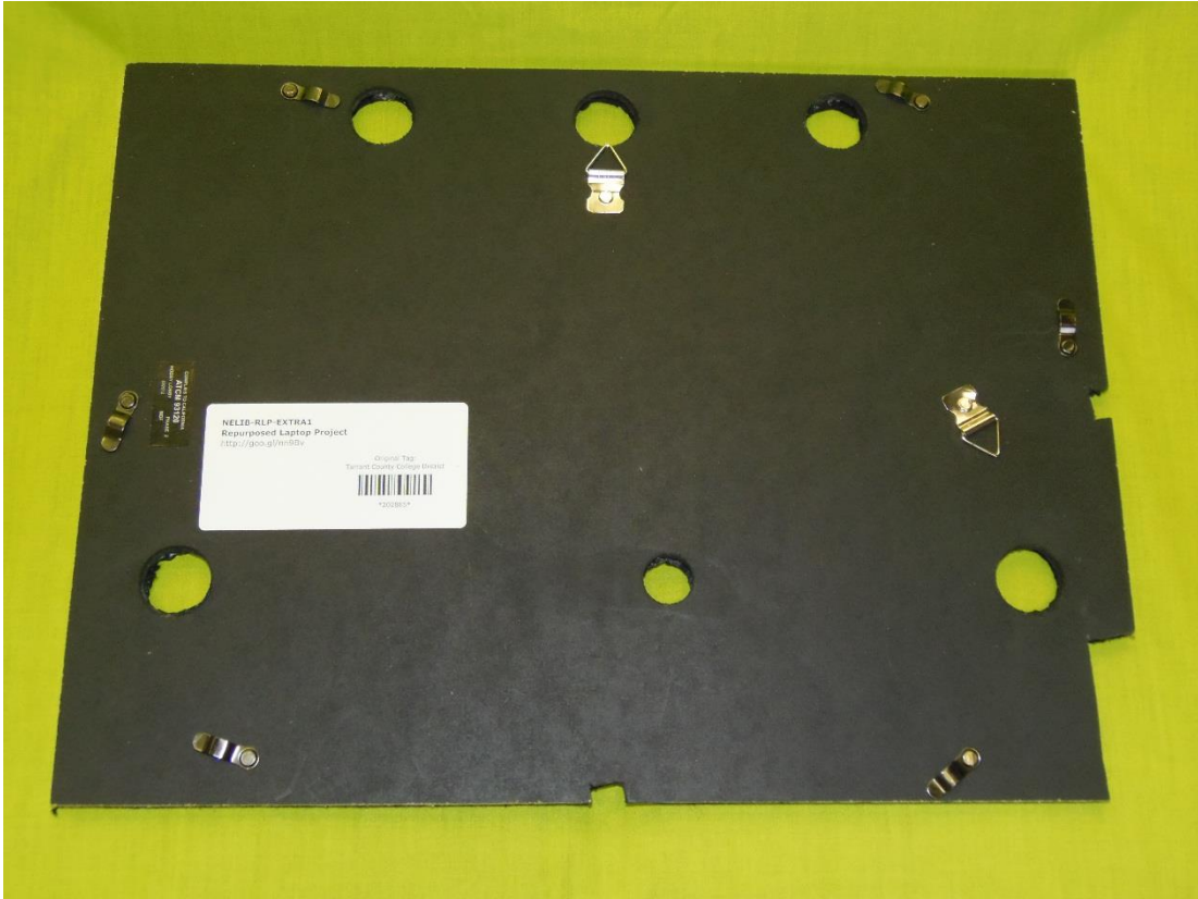
Figure 6. Holes in back cover for air circulation and power button.
