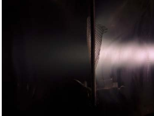
Figure 6.2. An optical photograph of the effects of placement of a floating stainless steel mesh 8 screen on the visible glow of Ar LTCAT discharge under the conditions of 1000 sccm Ar and 4 A arc current.
