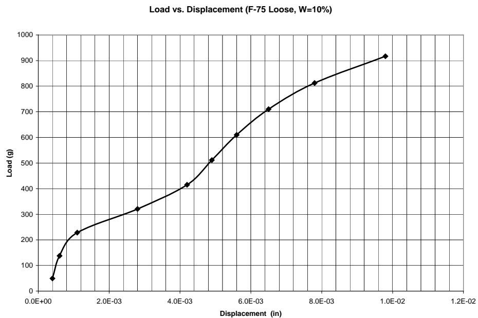
Figure B. 10: Load as a function of displacement in a tensile strength test for loose F-75 Ottawa sand ( e=0.75 and w=10\% )
