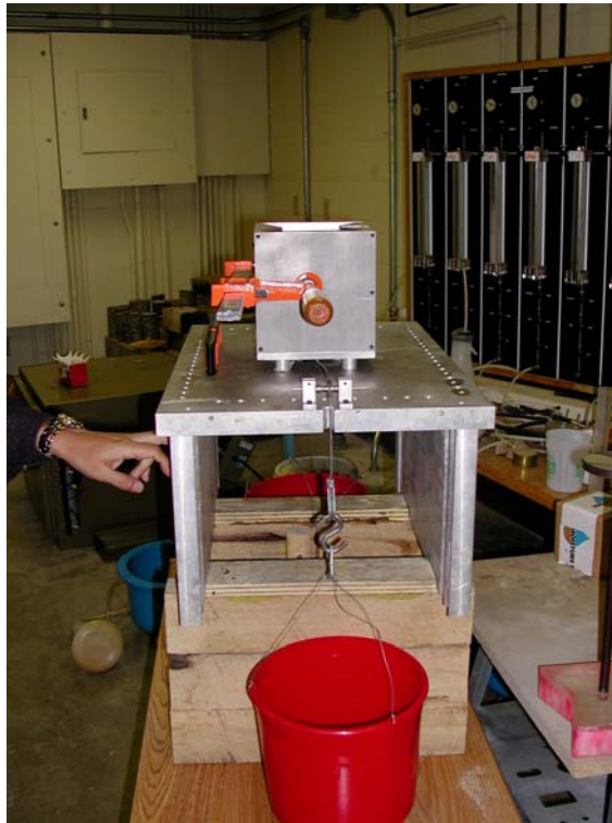
Figure 3. 27: Loading system used to apply tensile stress
