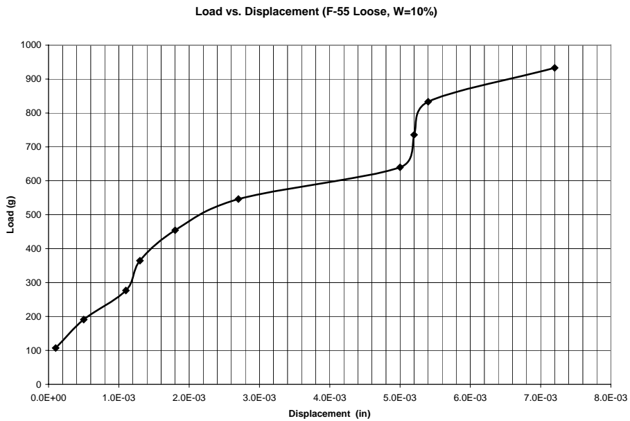
Figure B. 26: Load as a function of displacement in a tensile strength test for loose F-55 Ottawa sand ( e=0.75 and w=10\% )
