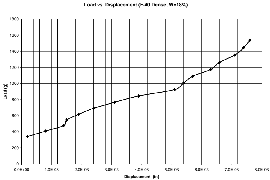
Figure B. 47: Load as a function of displacement in a tensile strength test for dense F-40 Ottawa sand ( e=0.60 and w=18\% )
