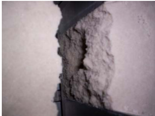
Figure 5. 42: Pattern of failure surface in a tensile strength test for dense F-75 sand ( e = 0.60 ; S = 80\% ). Capillary regime boundary
