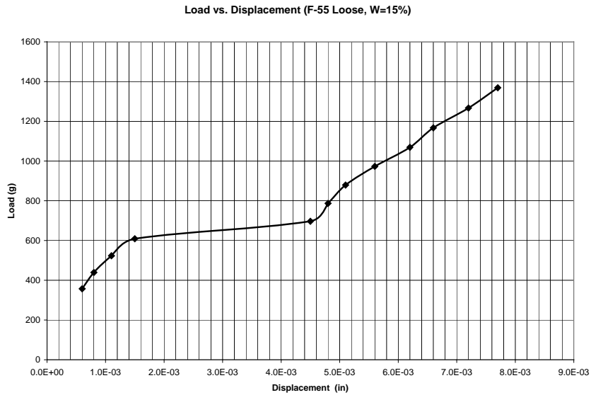
Figure B. 30: Load as a function of displacement in a tensile strength test for loose F-55 Ottawa sand ( e=0.75 and w=15\% )
