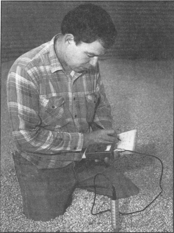
Figure 5. Monitoring and recording grain temperature with an electronic thermometer. You should probe several areas inside the bin for hot spots.
