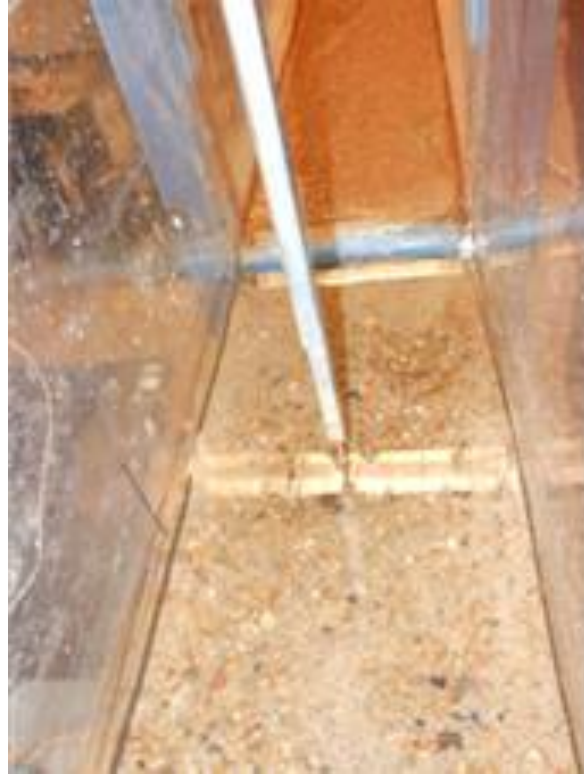
Figure 3.3 Photographic descriptions of major stages in each test. From top to bottom: structure stabilized in soil prior to water flow; induced surge event occurs; scour reconnaissance and measurements recorded [28]
