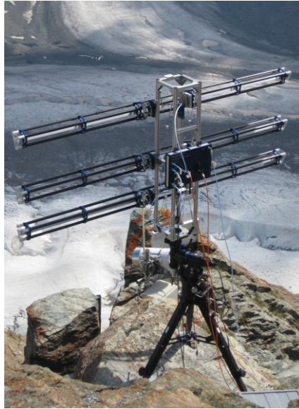
Figure 3.3 GAMMA Remote Sensing ground based system, GPRI-I (Werner, et al., 2009)
