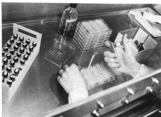
Technician is adding serum to wells for testing. The serum is taken from vials in the rack on the left.
