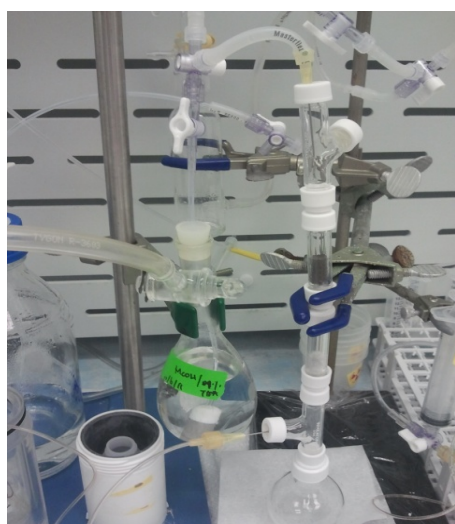
Figure 4-1. Picture of the reaction setup of reductant column connected to the separation column filled with a chromatography media. This setup uses a solvent reservoir to transfer the eluting solvent (EtOH/ACN) to the column.
