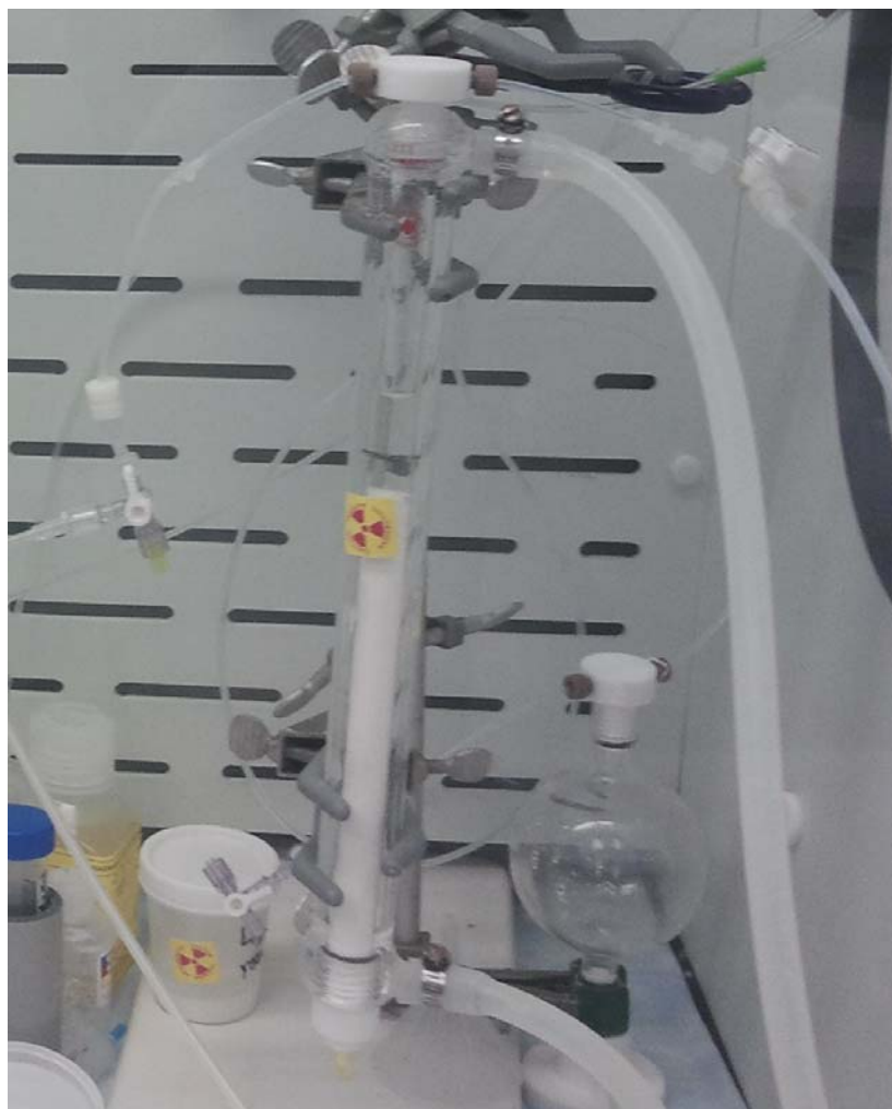
Figure A 3-7. Picture of column chromatography separation using Ln2 resin as extraction media with heat exchange jacket. The flow rate of the column is controlled by adjusting flow gauge of a compressed N 2 to obtain the desired flow rate.
