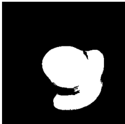
Serious over segmentation
