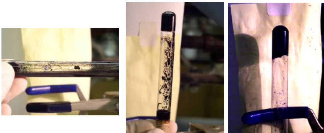
Figure 4.10. Solutions of macrocycle and nanotubes after one hour sonication. Left: An ungelled solution (Solvent: carbon disulfide). Center: A partially gelled solution, not liquid at bottom of vial on cork (Solvent: NMP). Right: A completely gelled matrix (Solvent: Hexane).
