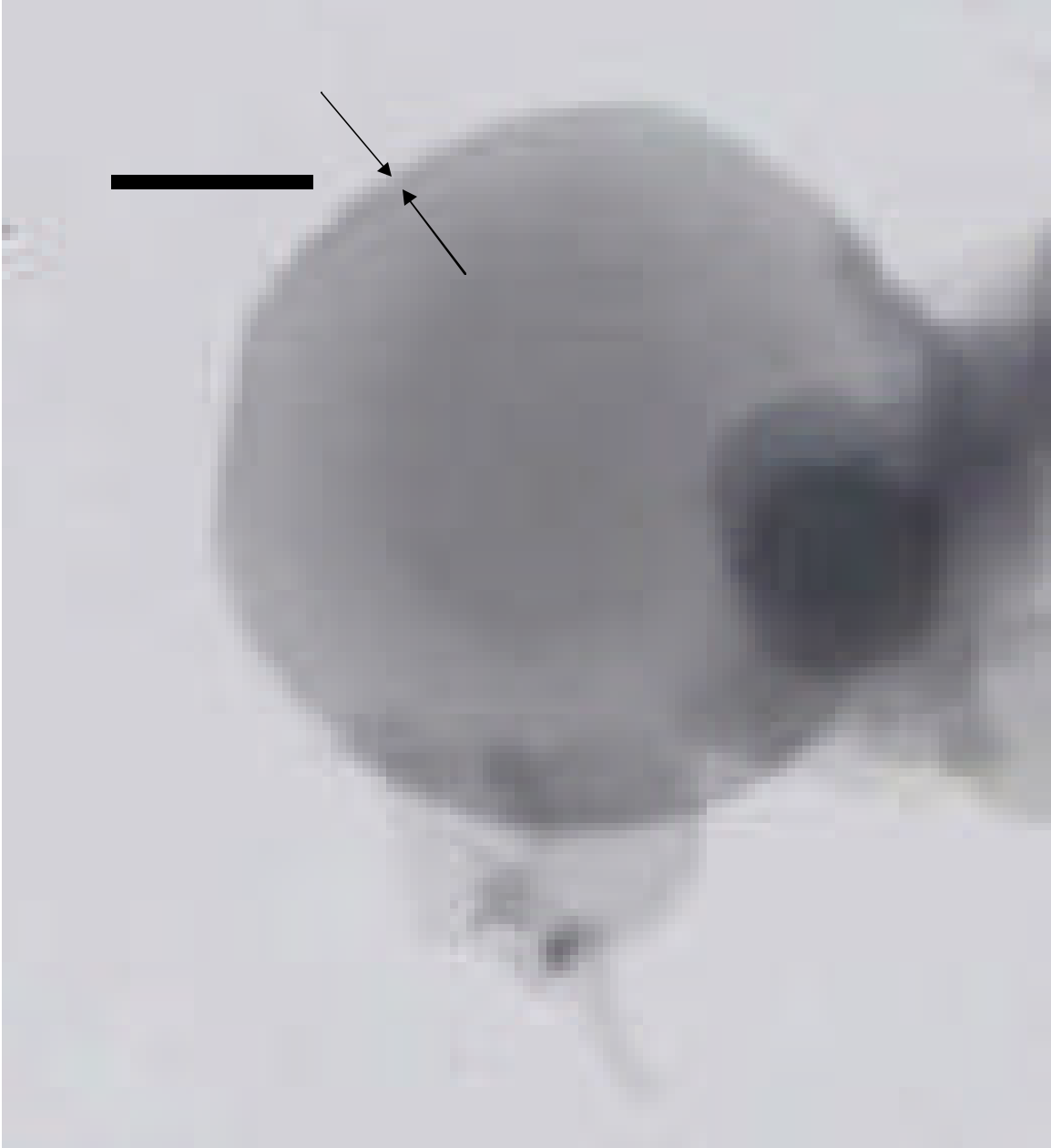
Figure 5.10. Blowup of left image in Figure 5.9. Some of the spheres seem to have a darker area around their edges, perhaps indicating the wall of the sphere. Estimates from this structure put the wall at about 4 nm thick (Scale bar = 100 nm).
