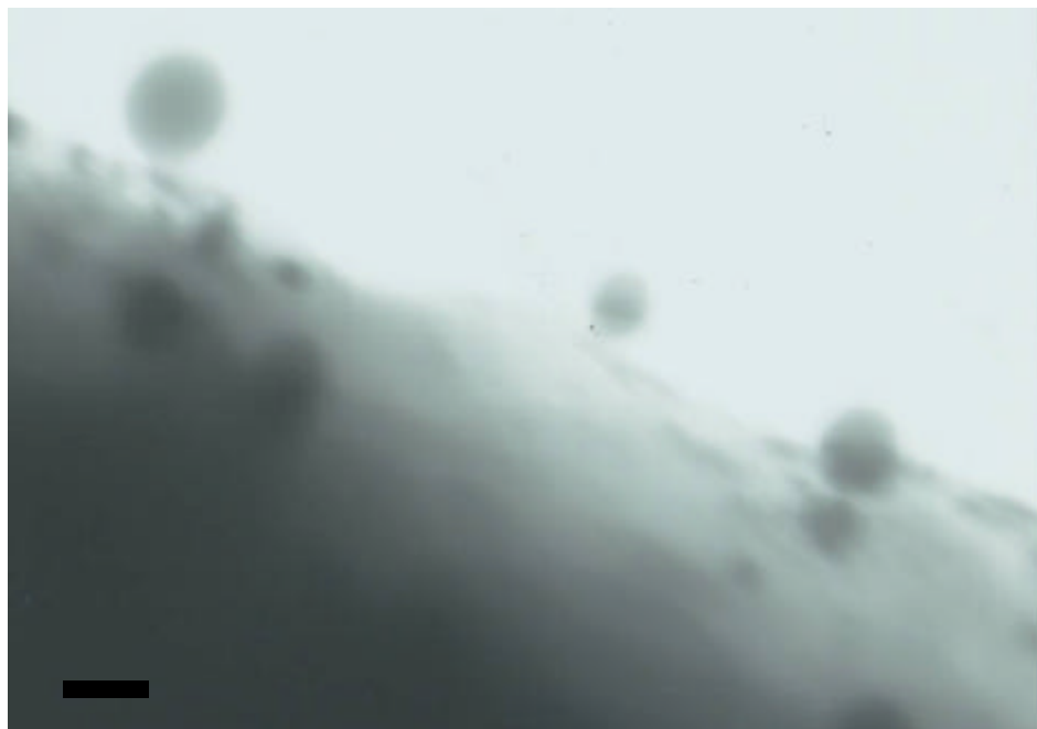
Figure 5.14. A tear in the carbon sheet of the TEM grid reveals spheres hanging to the edge of the sheet as it rolls around from the energy of the electron beam ( R = -C_3H_7 , Scale bar = 50 nm).
