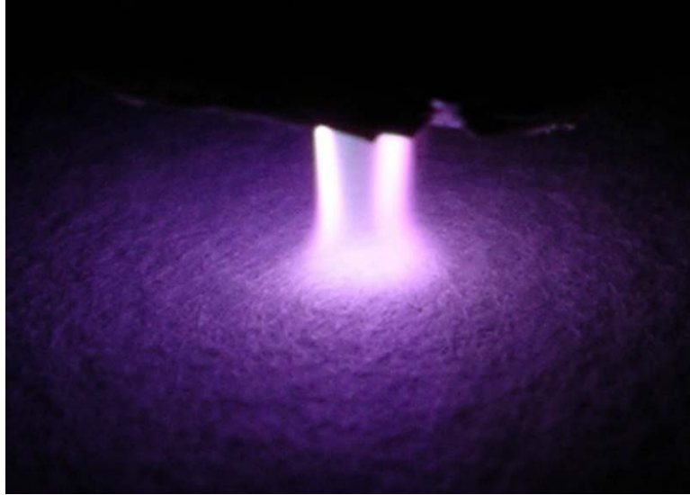
Figure 4. 1. Photographs of an argon atmospheric plasma brush touching a paper surface. Plasma conditions are 1500 sccm argon, 15 w DC power input.
