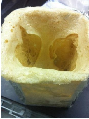
Figure 4.1 Collapse of the flexible polyurethane foam with no cross-linker content but 100% castor oil replacement.
