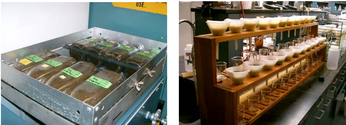
Figure 7.2. Reciprocating shaker (left) and filtering device (right) for soil nutrient extraction.
