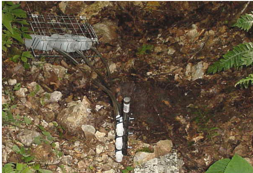
Figure 3.1 – Rising stage water sampler seen facing downstream.
