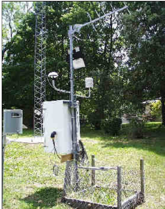
Figure 3.15 – Typical Remote Automated Weather Station (RAWS).
