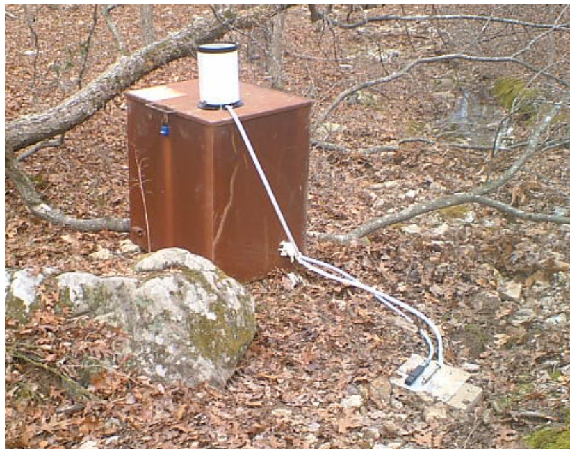
Figure 3.6 – Isco® automatic water sampler installed in security box.
