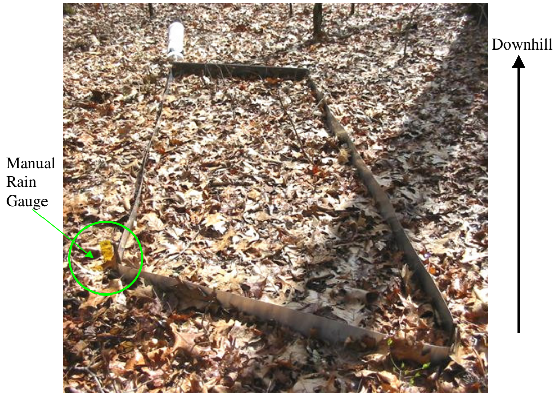
Figure 3.10 – Hillslope sediment monitor and manual rain gauge.
