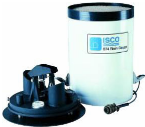
Figure 3.9 – Isco® 674 rain gauge.
