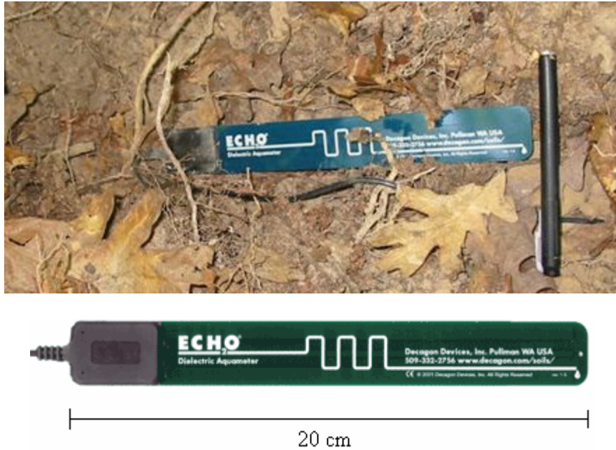
Figure 3.17 – ECH2O® EC-20 soil moisture probe.
