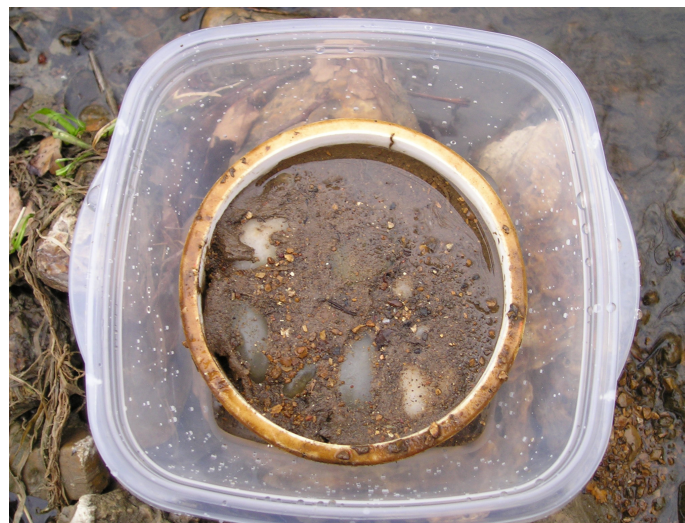
Figure 5.—Photographs that show the installation of a deposited-sediment sampler in the streambed (top and middle) and the collection of a sampler with the bottom-insert cap removed (bottom).
