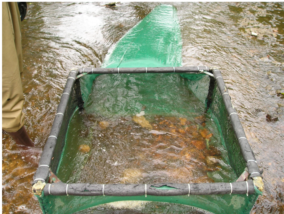
Figure 6.—Photograph of the 1-m 2 quadrat sampler used to sample benthic fishes in riffle and run mesohabitats. Notice the collection bag on the downstream side of the sampler.
