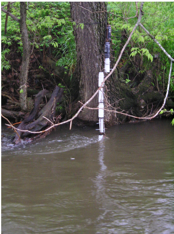
Figure 3.—Photograph that shows the single-stage bottle sampler arrangement at one study site during the rising limb of the hydrograph. Some bottles were painted black.
