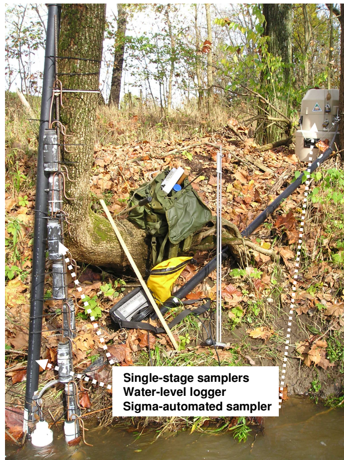
Figure 4.—Photographs of the procedure for measuring stream discharge along a transect at site 6 (top) and the sampling and measuring equipment at site 7 (bottom).
